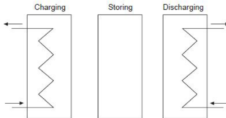
Figure 1: Storage cycle of TES system (Cabeza, et al., 2015)
