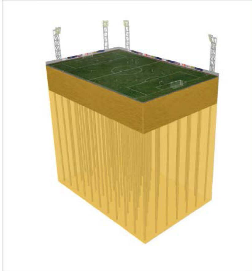
Figure 7: Example of borehole field that has a football field on top of it (Wincott, 2011)
