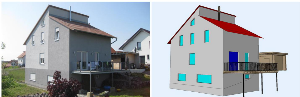
Figure 11. Example of a building modeled in LOD3 (OGC 2012).
