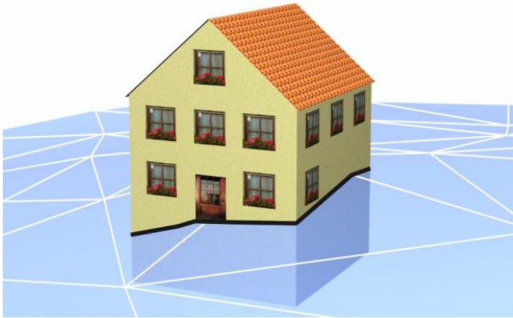
Figure 18. Example of the Terrain Intersection Curve represented as black line (OGC 2012).
