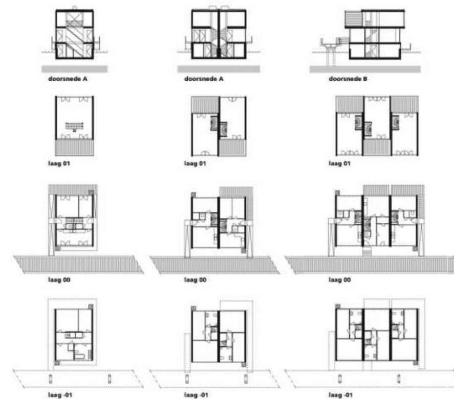
Figure 9. Picture showing the different variations in apartment sizes build from modular parts.
