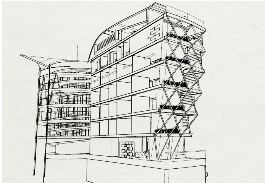
Figure 55. Section from the apartment block showing the modularity, façade and the pedestrian spiral ramp
