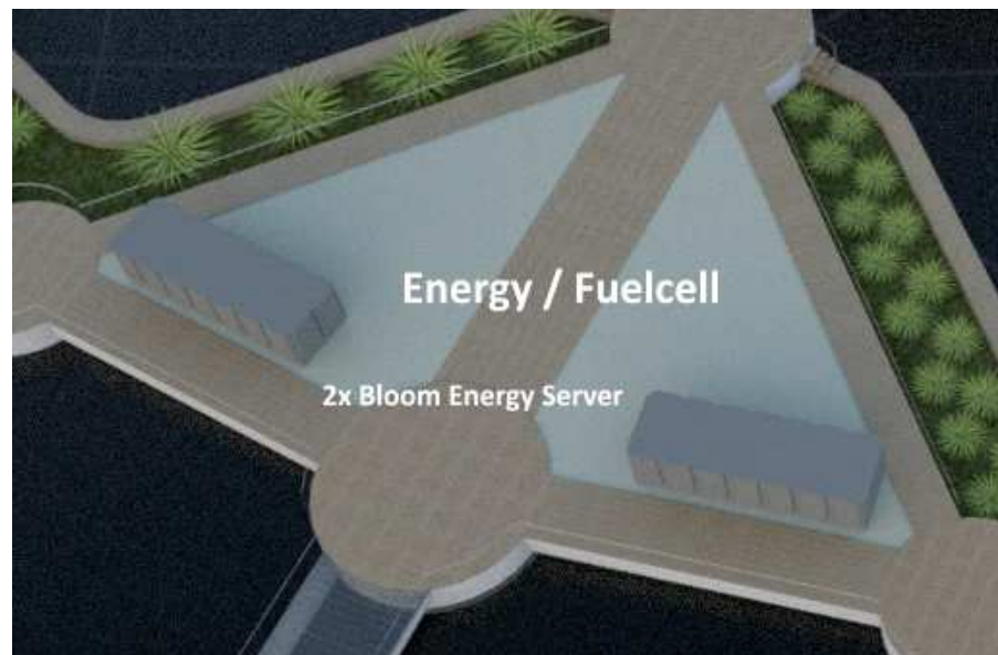
Figure 61. Rendering showing the Bloom Energy servers situated near the main walkway for maintenance reasons.
