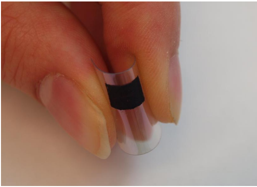
Figure 2. Bending of a counter electrode consisting of carbon gel catalyst layer on ITO-PET.
