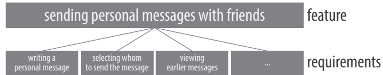
Figure 1. A feature represents a logical unit of behaviour from the stakeholder’s perspective
