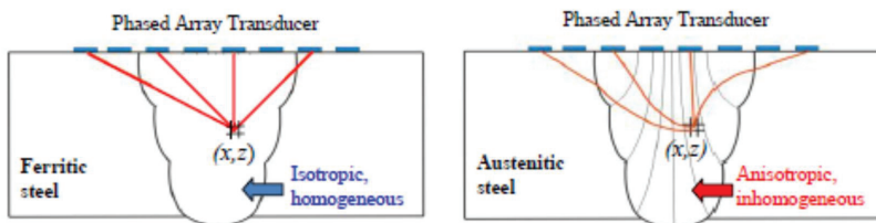
Figure 9. Schematic comparison of sound paths for computation of propagation times in ferritic and austenitic steel [10].
