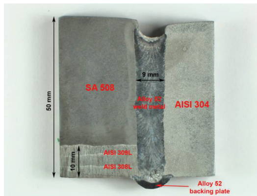
Figure 4. A modern NG DMW safe-end design.
