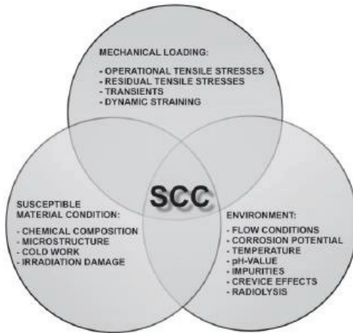
Figure 3. Critical factors for stress corrosion cracking. [2]
