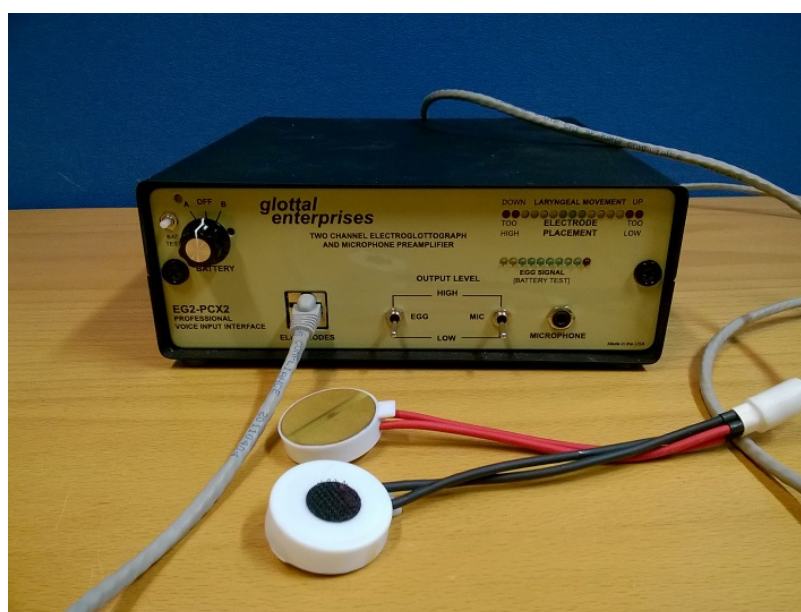
Figure 11: Electroglottograph pre-amplifier and electrodes
