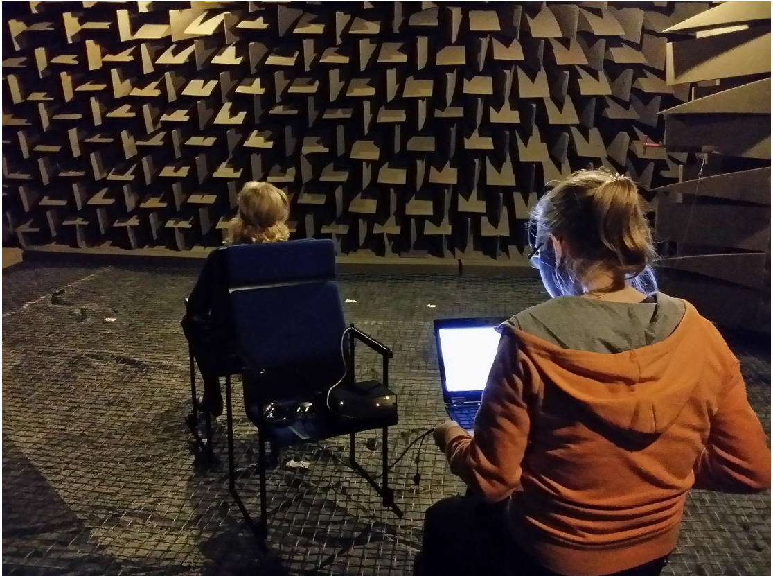
Figure 15: The subject (behind) is reading while the experimenter (in front) is monitoring the signals. The sound card and EGG pre-amplifier are placed on the chair next to the experimenter. Photographer: Christoffer Kauppinen
