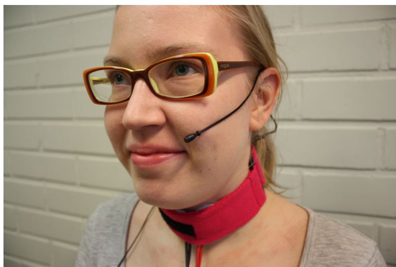
Figure 13: EGG electrodes and microphone on a speaker
