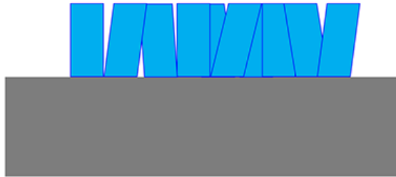
Figure 15: Columnar and mosaic film on substrate, illustrating the tilt of the columns, which leads to peak broadening in XRD.
