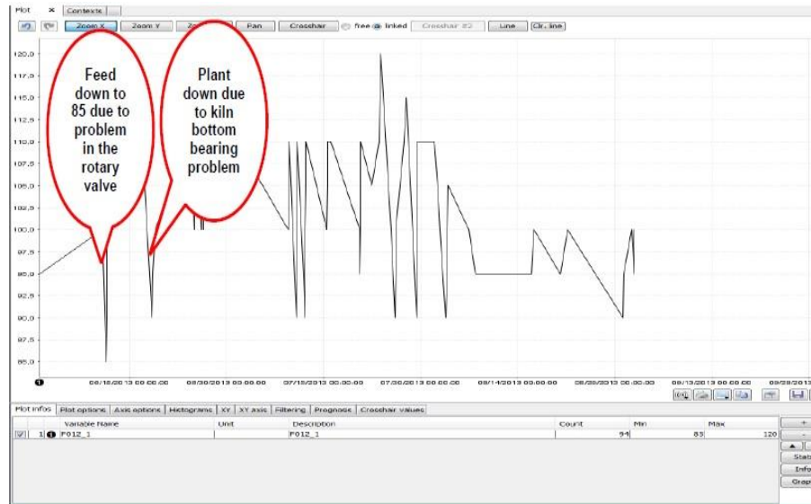
Figure 7.2: Visualizing the effect of rotary valve problem and plant shutdown on the feed rate
