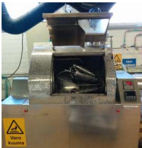
Figure 21. "Muru" air bath digester.
