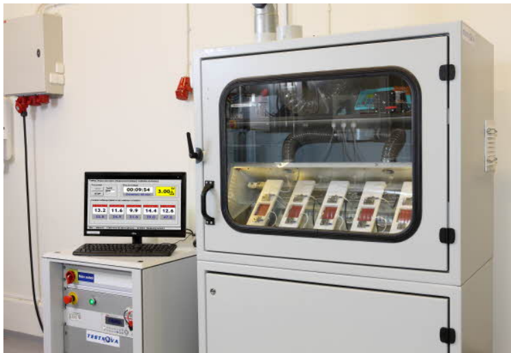
Figure 24: Test chamber for the inclined plane test
