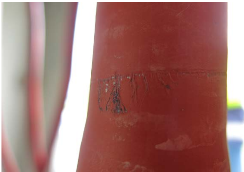
Figure 10: Anaerobic tracking paths under a loose rain shed in a heat-shrink termination
