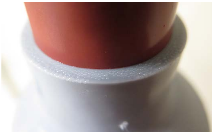
Figure 29: Water droplets on the edge of the rain shed
