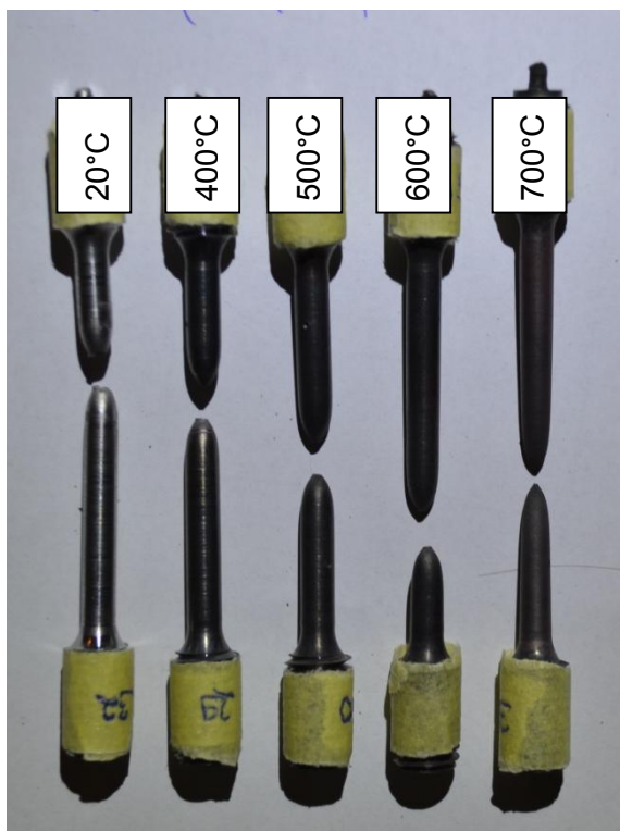
Figure 4.13 S700QL, steady state tests failure modes
