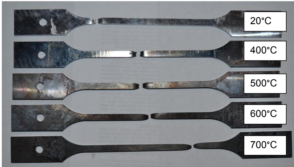
Figure 4.12 S960QC, steady state tests failure modes
