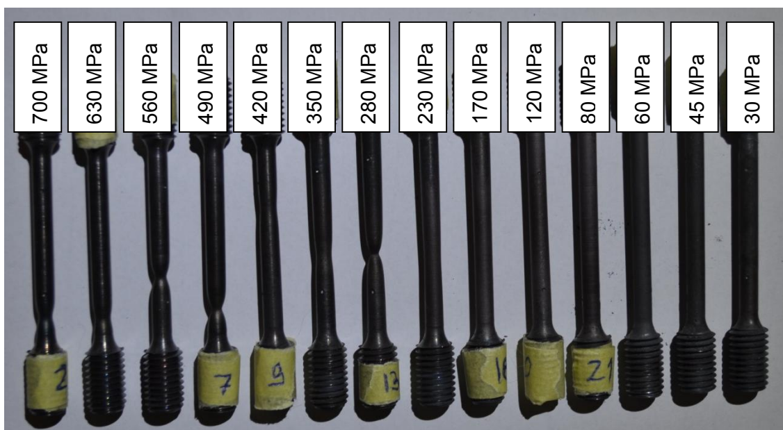
Figure 4.11 S700QL, transient state tests failure modes
