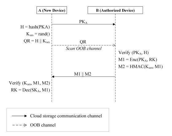
Figure 4.4: Key distribution using QR code
