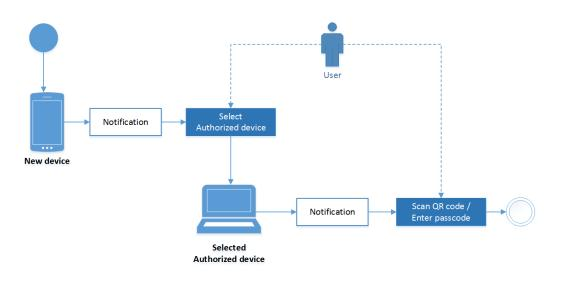
Figure 6.4: Work flow for device authorization from user perspective
