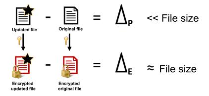
Figure 4.7: Encryption does not keep the update difference.
