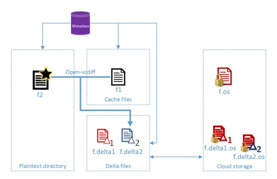
Figure 5.7: Incremental synchronization implementation
