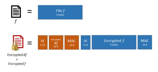
Figure 5.2: Format of an encrypted file
