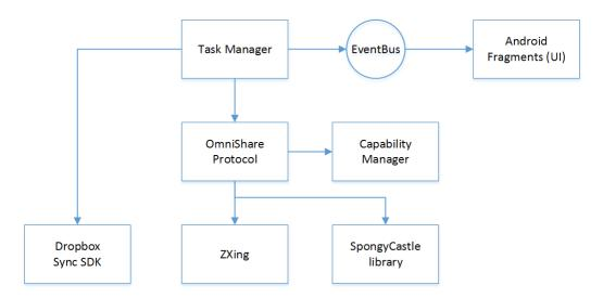
Figure 5.4: Software architecture of OmniShare on Android
