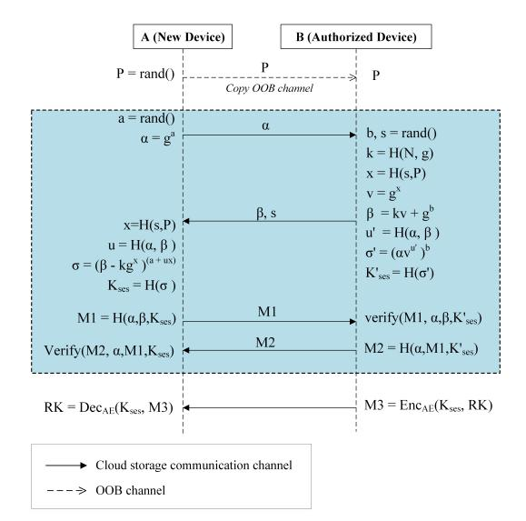
Figure 4.6: Key distribution using SRP
