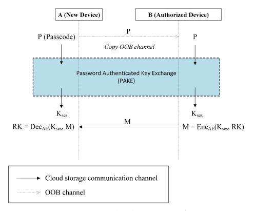
Figure 4.5: Key distribution using PAKE
