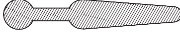
Fig. 2: Cross-section of a rotor bar. Diameter of the rotor is 198 mm and height of the rotor slot is 35 mm.
