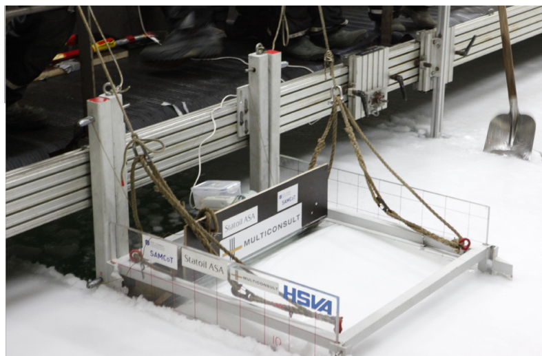
Figure 7: The model is pushed into the intact ice from the left in an experiment carried out in reverse-motion mode. (Image by courtesy of Wenjun Lu.)
