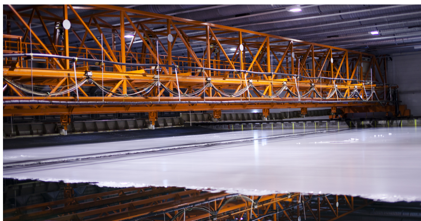
Figure 6: Model scale experiments are conducted in special facilities called model ice basins. The Aalto Ice Tank is a large model basin where Arctic ice conditions can be simulated. (Image by the courtesy of Aalto University.)
