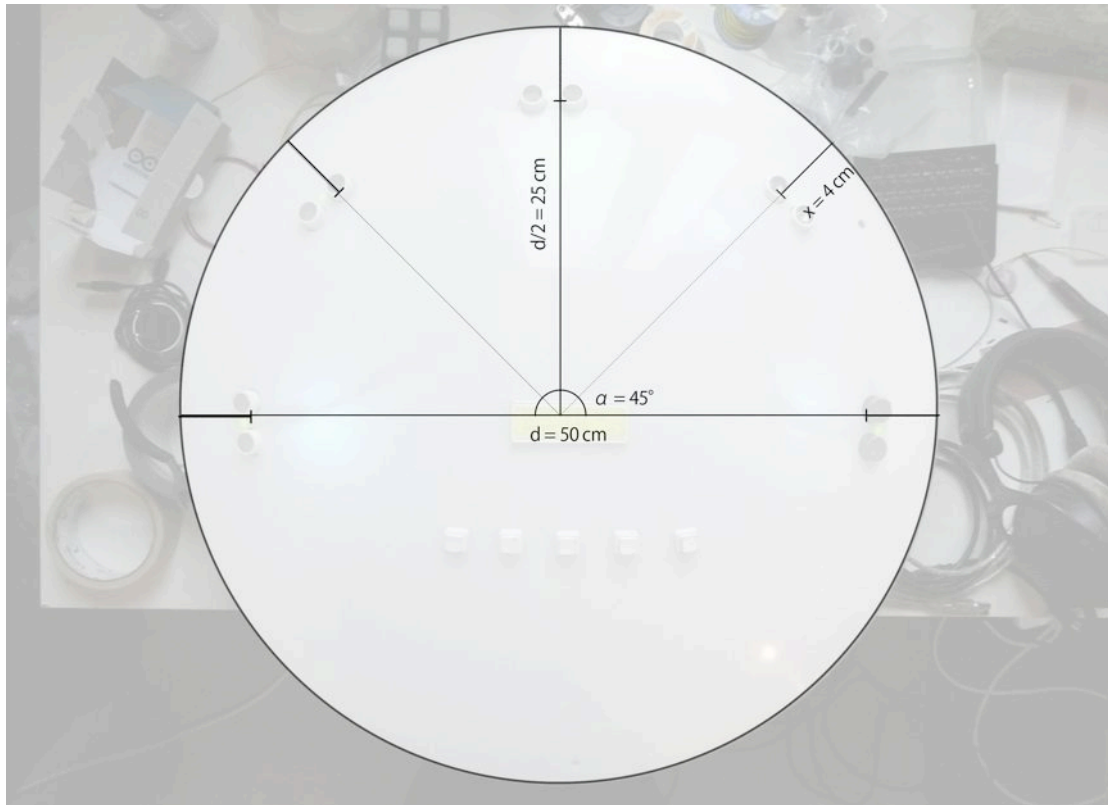
Figure 9. Even distribution of the five ultrasonic sensors in a semicircle ( d = diameter, x = distance of the sensor from the outer edge of the device).
