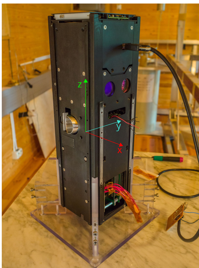
Figure 8: Aalto-1 engineering model with the spacecraft body reference frame definition.
