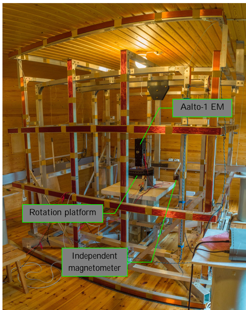
Figure 22: The magnetic test facilities with Helmholtz cage setup in Nurmijärvi Geophysical Observatory, operated by Finnish Meteorological Institute. The specifications of the test setup are available in [27].
