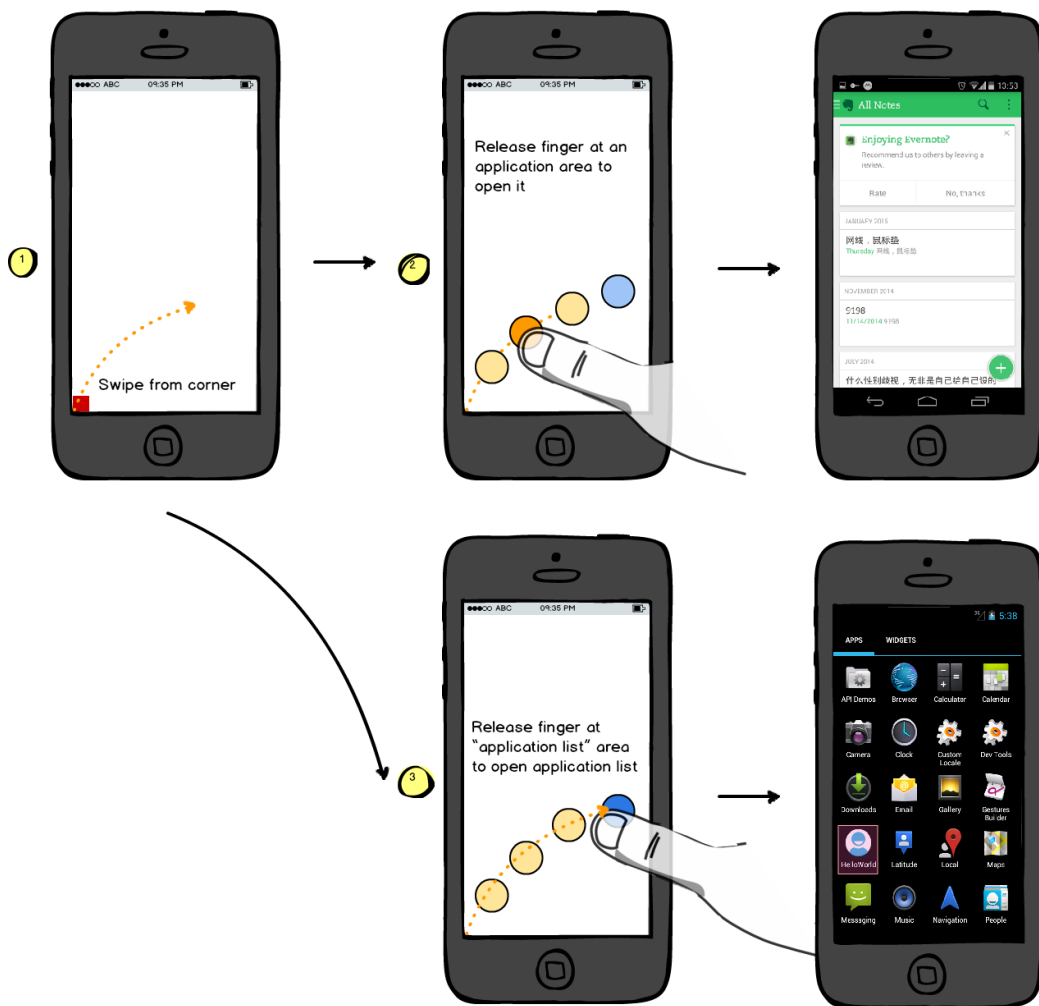
Figure 6.4: Workflow of SwipeLauncher section
