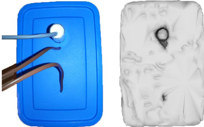
Figure 19 The photograph of the phantom from above, and a binary mask created with FSL, which shows the part of the phantom containing agar. Pipe with grey wire is the heating device. Brown wires are the T-type thermocouples measuring the temperature.
