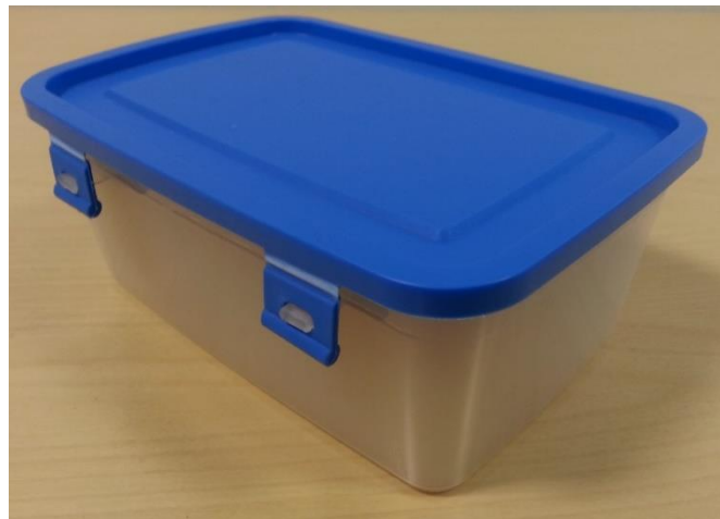
Figure 10 An example of one of the phantoms build for thermometry purposes. Phantom is plastic lunch box filled with agar gel.
