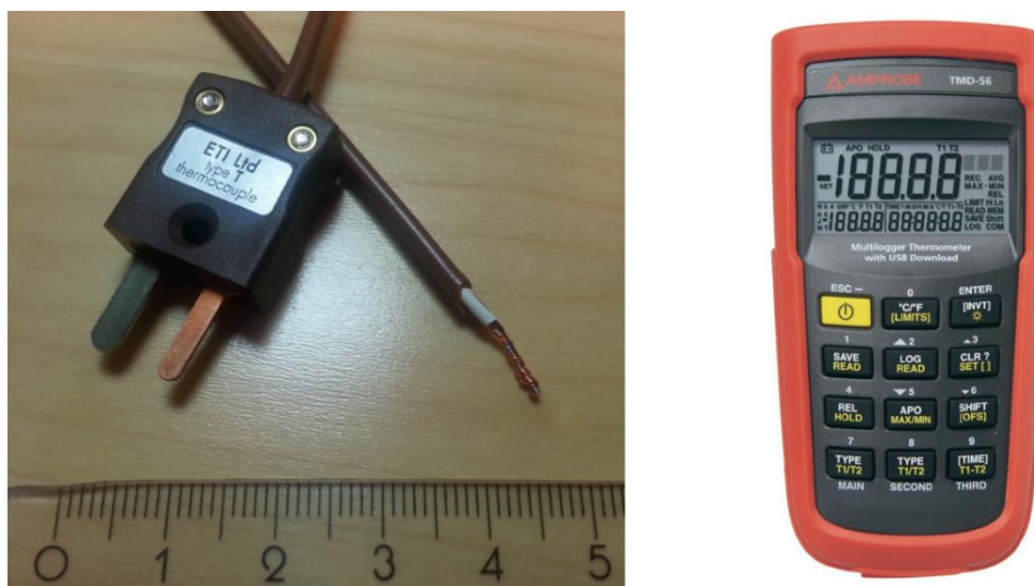
Figure 11 T-type thermocouple and Amprobe TMD-56 thermometer used in the thermometry studies. The exposed wires at the tip of the thermocouple were finally coated with thin plastic sock. Notice that the wires and corresponding connectors are made from same metal.
