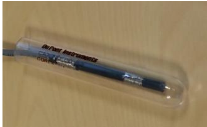
Figure 12 The tip of the heating device before it was filled with silicon glue and infused in to the agar phantom
