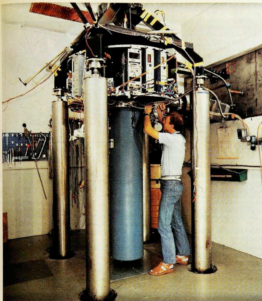
ROTA laboratory at the Helsinki University of Technology in Espoo, Finland. The rotating cryostat is supported on the four pillars at the center of the photo. Graduate student Kaj Nummilla is preparing the cryostat for rotation by disconnecting the external pumping lines. Figure 1
