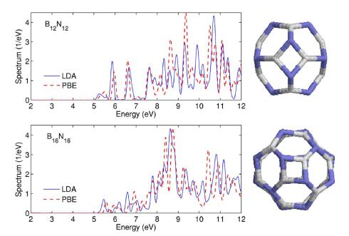
FIG. 1. (Color online) Photoabsorption spectra of  $\rm B_{12}N_{12}$  and  $\rm B_{16}N_{16}$ . The insets on the right-hand side show the optimized structures of the molecules.
