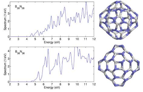
FIG. 3. (Color online) Photoabsorption spectra of  $B_{28}N_{28}$  and  $B_{36}N_{36}$ . The insets on the right-hand side show the optimized structures of the molecules. LDA approximation has been used.
