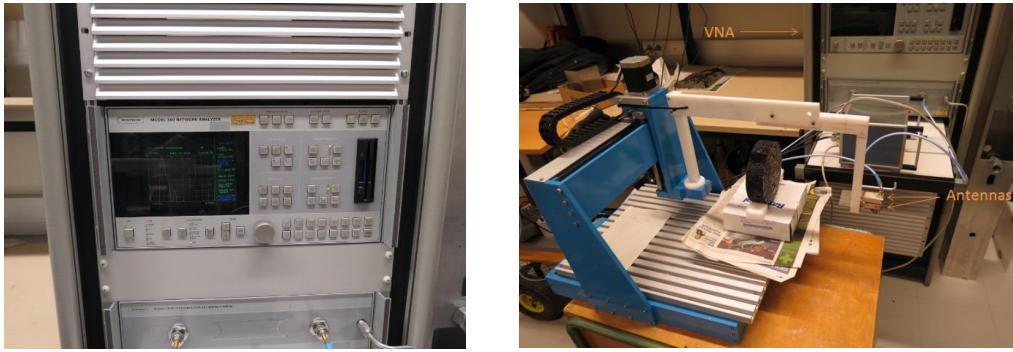
Figure 38. a) VNA apparatus, (b) core sample measurement set up on the right.
