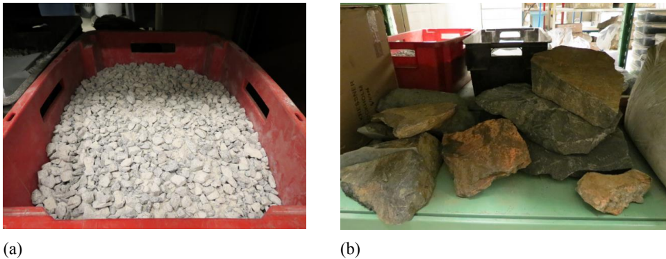
Figure 36. a) Blended aggregate without bitumen and fibers. b) Rocks collected from Mäyry quarry
