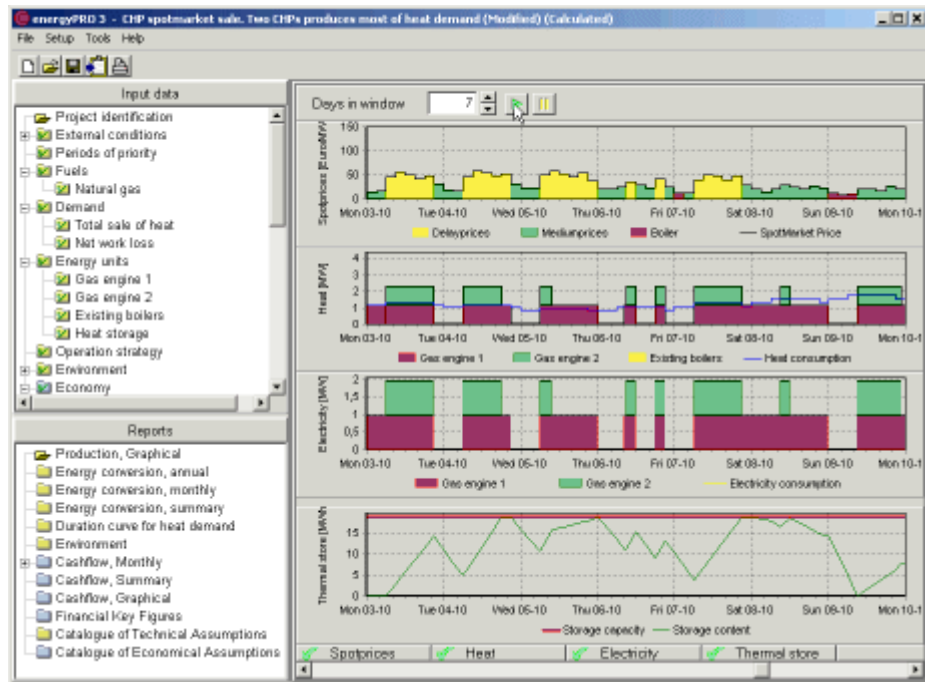
Figure 15. Example of how the results are shown hourly in graphical format in the energyPRO simulation tool (EMD International A/S, 2013)
