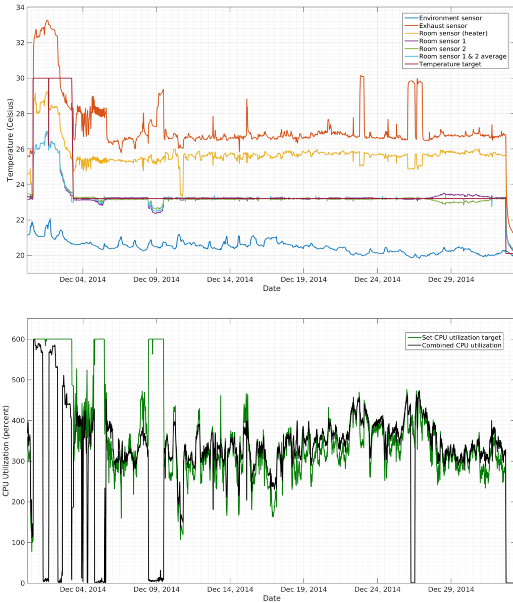
Figure 4.4: Temperature control test 2: December 3rd-January 7th. As we can see, the prototype can control the temperature in new environment very well, provided that suitable workload is available.
