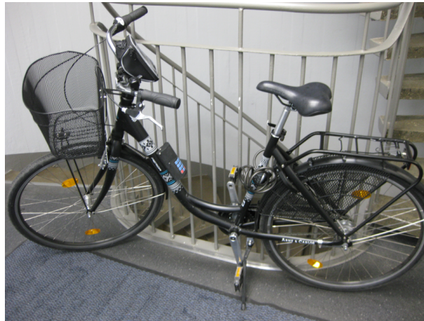
Figure 5.2: The second iteration bike lock, Viola, mounted on a woman's city bike. It was one of two bikes used for the internal testing.
