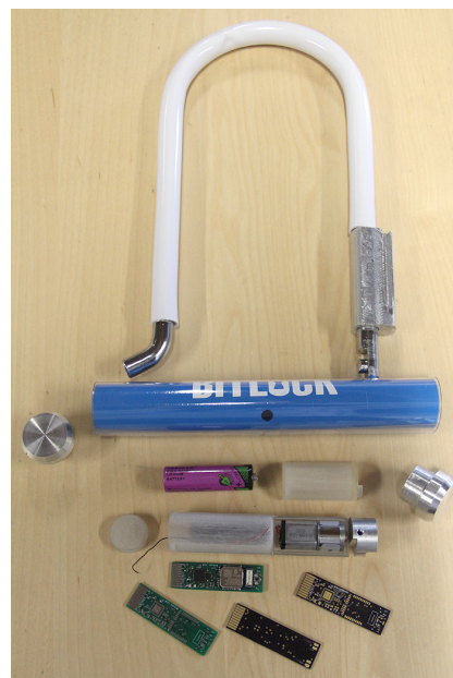
Figure 2.5: The BitLock and its electronics[29].
