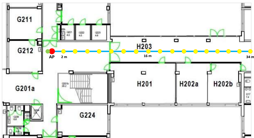
Figure 19: Testbed area including the location(s) of the AP (red dot) and the stations (green and yellow dots). (Figure not drawn to scale).
