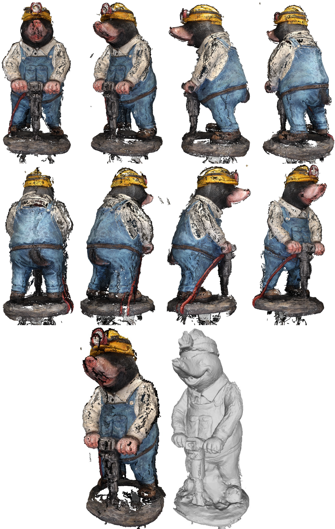
Figure 57: A full statue as a 360-degree point set, combined in Meshlab from four scans, and meshed. A slight misalignment between two of the clouds is visible. Misalignment errors could be addressed by more careful alignment and outlier removal, or a bigger rig with more cameras.
