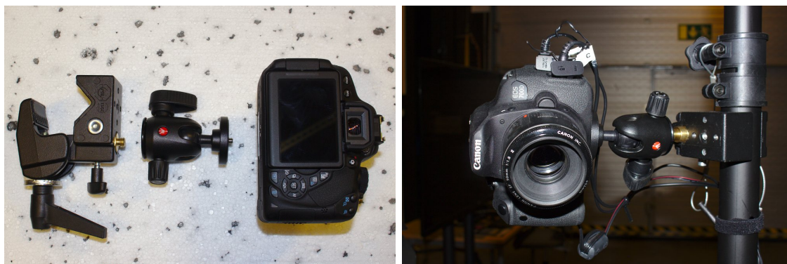
Figure 31: Left: the Super Clamp, ball head, and a camera separately. Right: one camera connected to the pole and its wires.
