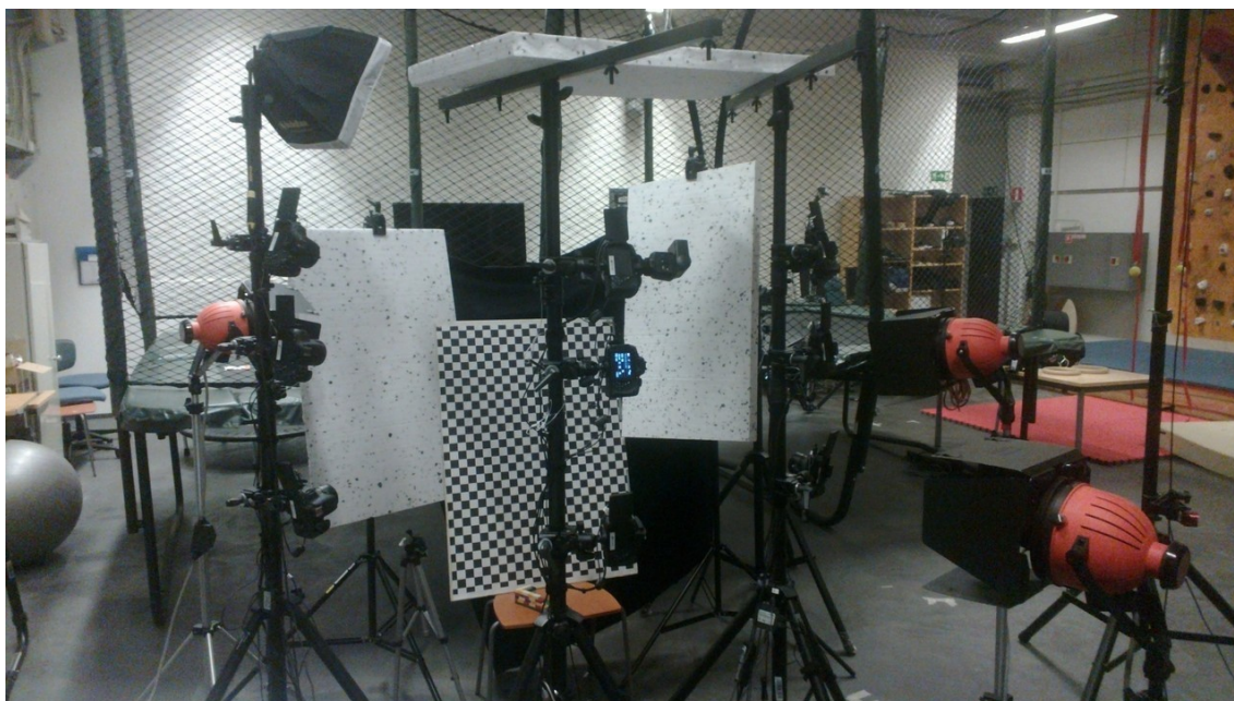
Figure 32: Complete setup with cameras and spot lights for video recording. In typical scans, the cameras would be slightly closer to each other.
