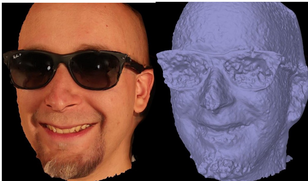
Figure 59: PhotoScan reconstruction from video frames, textured and solid. The solid rendering shows the relatively low vertex count and high amount of spatial noise, which are hidden in this particular textured demonstration view.
