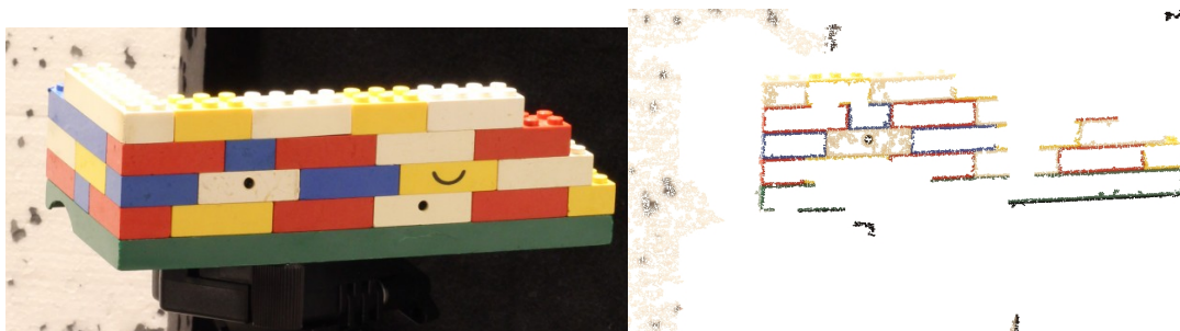
Figure 58: A lego block structure demonstrates that textureless surfaces reconstruct poorly, as was expected. The old and dirty block in the middle had enough texture to fill better than the others.
