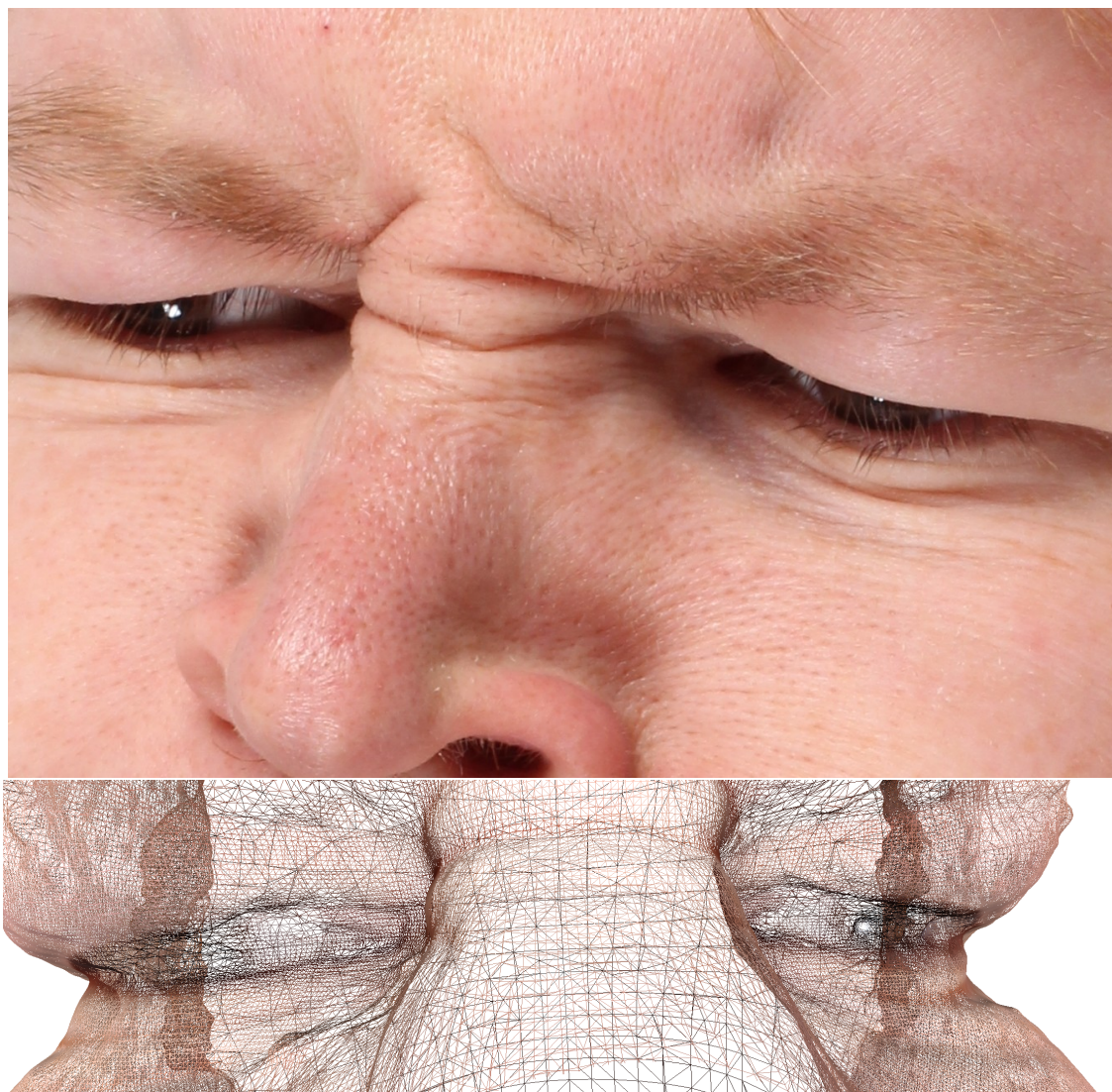
Figure 54: Close details from one camera, showing the mesoscopic level of detail, and a corresponding area as a transparent wireframe mesh, showing the amount of vertices. Note that the mesh does not yet employ the full geometric properties of the source photograph, i.e., the pores and wrinkles, that are beyond the geometric detail of the mesh.
