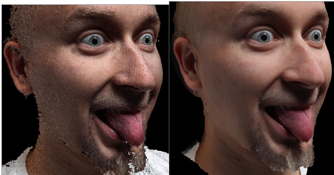
Figure 49: A dense point set (left) and a textured mesh in PhotoScan, matching the pictures in Figure 48. The underlying triangle mesh contains as much noise as the point set, which is hidden by the noiseless texture.
