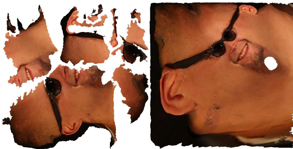
Figure 51: The “generic” (left) and “spherical” (right) texture mapping modes in PhotoScan. The missing spot under the chin is a result of poorly set up cameras that should have been set lower for more visibility.
