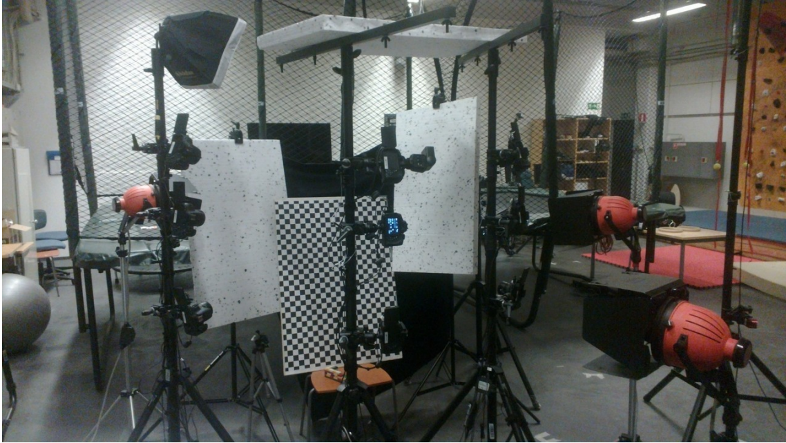
Figure 46: Complete setup with cameras mounted on the stands, surrounded by 800 watt spot lights (red) for video recording tests. For photos, the cameras were closer to each other as shown in Figure 47.
