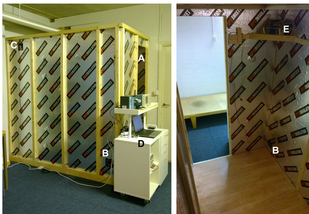
Figure 2 External (left) and internal (right) view of the test shed: (A) test shed entrance, (B) feeding and (C) exhaust air fans of the ventilation, (D) data acquisition equipment, and (E) radar sensor.
