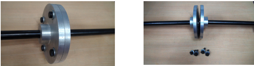
Figure 3. View of the cracked shaft (a) Joined by the four bolts (b) Disjoined
