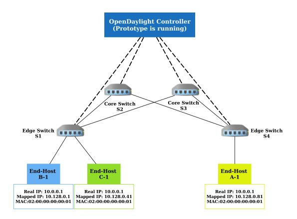
Figure 6.5: Test network for inter-tenant communications
