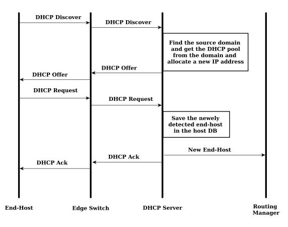
Figure 5.4: Host detection using the DHCP server
