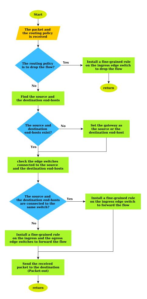
Figure 5.6: Reactive forwarding using the routing manager at the edge of the network
