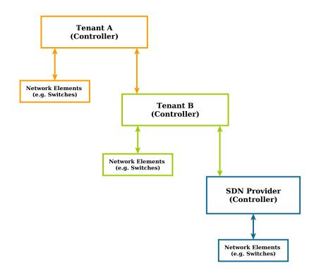
Figure 3.4: SDN Provider with Recursively Connected Tenant Controllers
