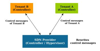
Figure 3.5: Packet rewriting at the controller plane
