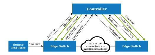
Figure 6.19: Control messages (OpenFlow) for processing a new flow request in our prototype
