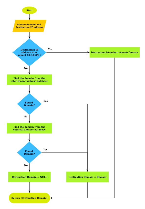
Figure 5.3: Implemented algorithm for finding the destination domain
