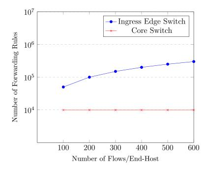
Figure 6.18: The number of flow entries at the ingress edge switch and the core switch
