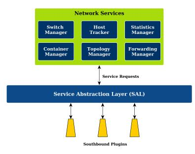
Figure 2.2: Service Abstraction Layer in the OpenDaylight controller
