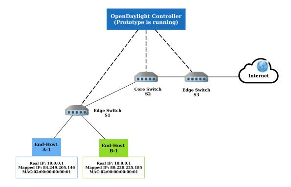
Figure 6.10: Test network for external communications
