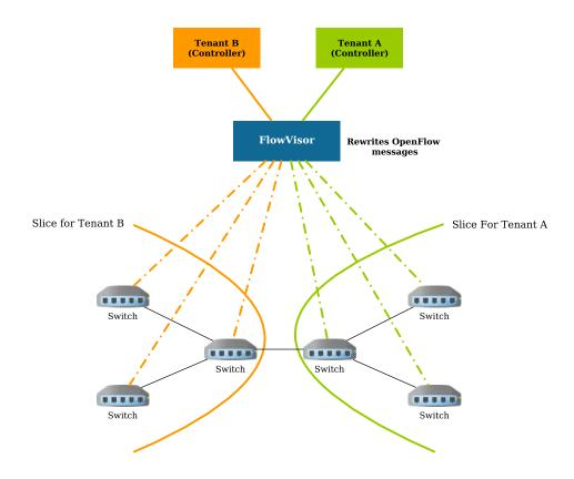
Figure 3.8: Slicing approach (topology slicing) in FlowVisor
