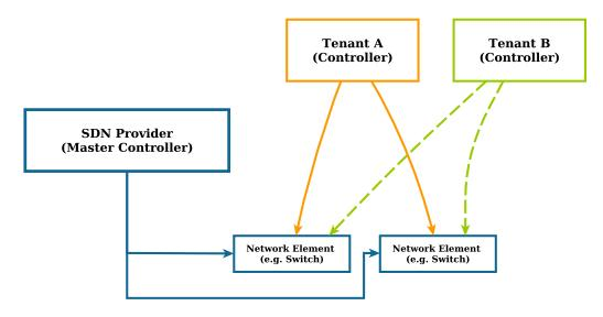
Figure 3.2: SDN provider with SDN tenants connected directly to the data plane
