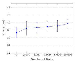
Figure 6.21: The latency of rule matching technique for installing forwarding rules
