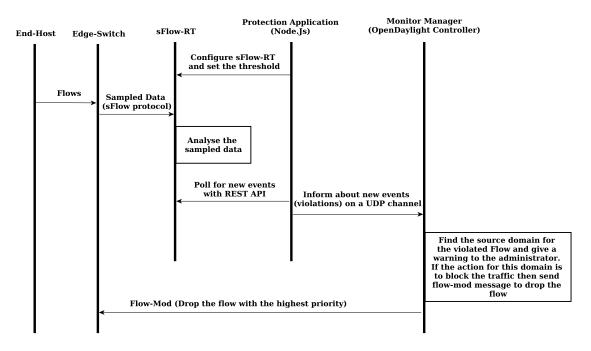
Figure 5.7: Message diagram for monitoring process in the prototype
