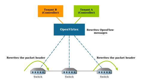
Figure 3.10: Isolation at the controller and data planes in OpenVirtex
