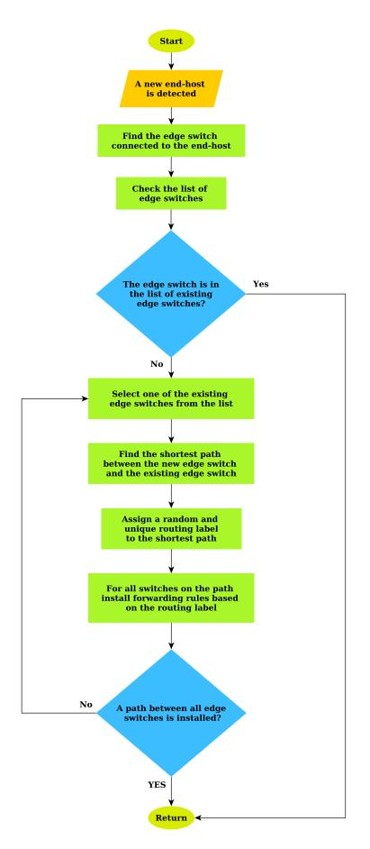
Figure 5.5: Proactive rule installation at the core network
