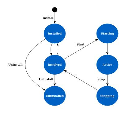
Figure 5.1: The operational states of a bundle in the OSGi framework
