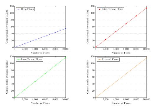
Figure 6.20: The amount of control traffic based on the number of new flow requests (a) dropped, (b) intra-tenant, (c) inter-tenant and (d) external communications
