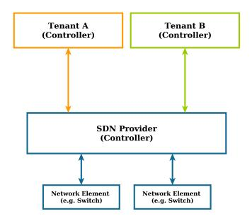
Figure 3.3: SDN Provider with Non-Recursively Connected Tenant Controllers
