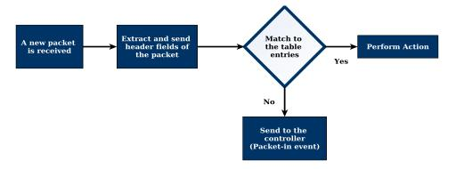
Figure 2.3: Simplified diagram of flow matching in an OpenFlow-enabled device
