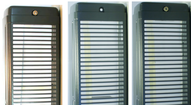
Figure 76. vPC samples after 6 months outdoor exposure. Samples from left to right: an unexposed sample and the samples tested in Oulu and Espoo.
