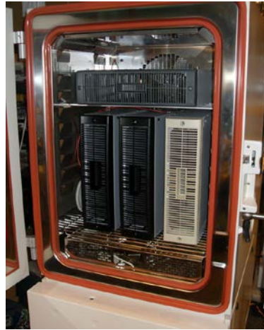
Figure 41. The test configuration for change of temperature test in Vötsch VC 3 7018 climate chamber.
