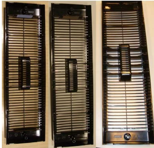
Figure 91. No visual changes were observed in rPC 30B cover after 0 (on left), 1000 and 2000 h in accelerated aging testing.
