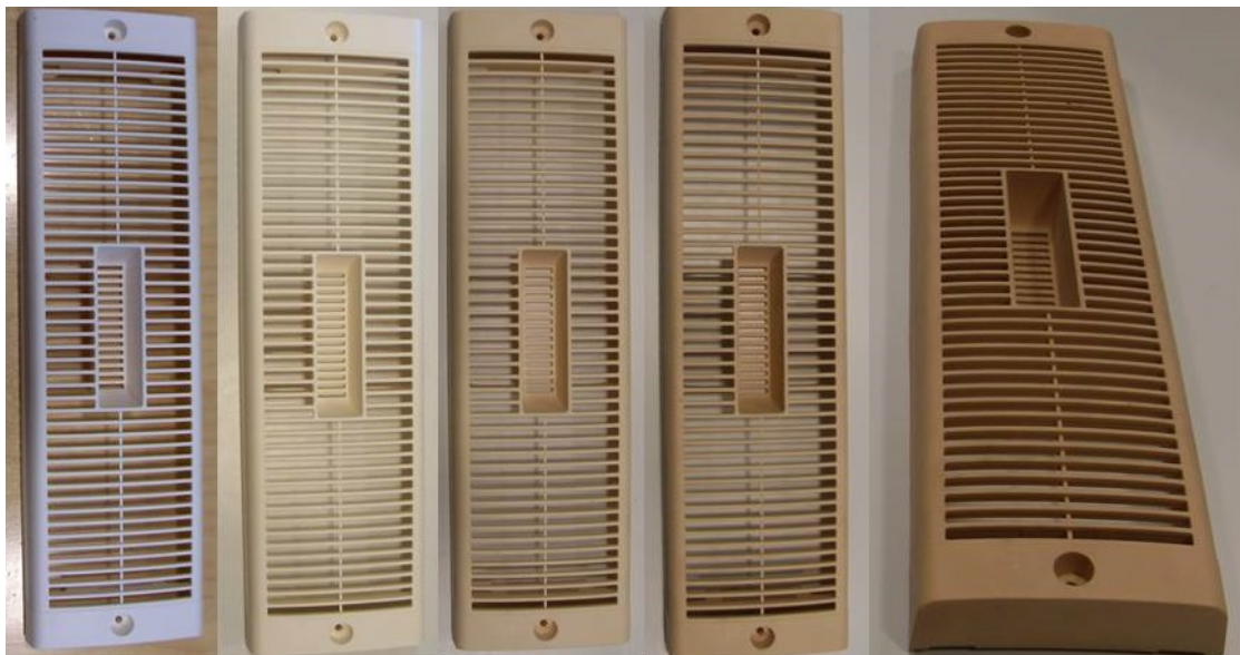
Figure 43. The colour change in PA410 in the accelerated aging testing. Photos were taken with digital camera after 0 (on left), 500, 1 000, 1 500 and 2 000 h.
