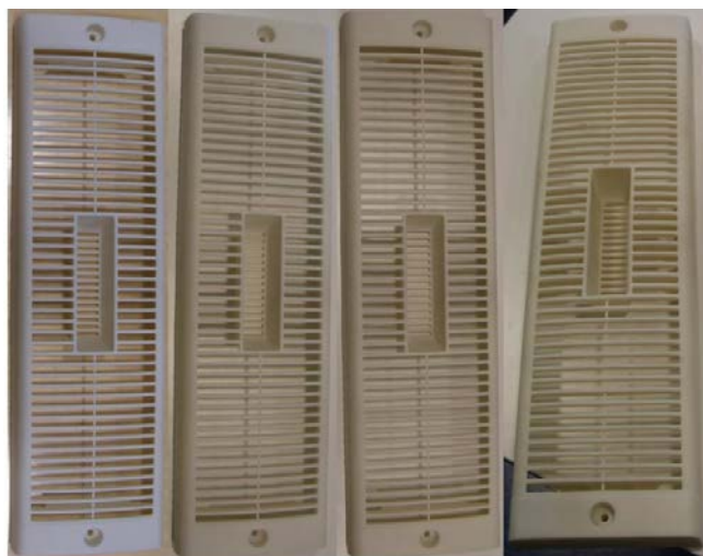
Figure 87. Visual inspection of PTT covers in accelerated aging testing after 0 (on the left), 500, 1000 and 2000 h. Colour of the cover became slightly lighter during the test.
