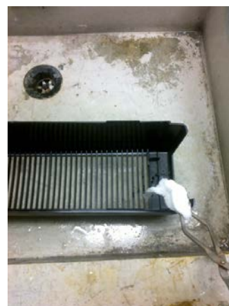
Figure 31. Configuration of the chemical testing: exposure by spraying and rubbing with cotton plug. Exposure times were 15 - 20 s.
