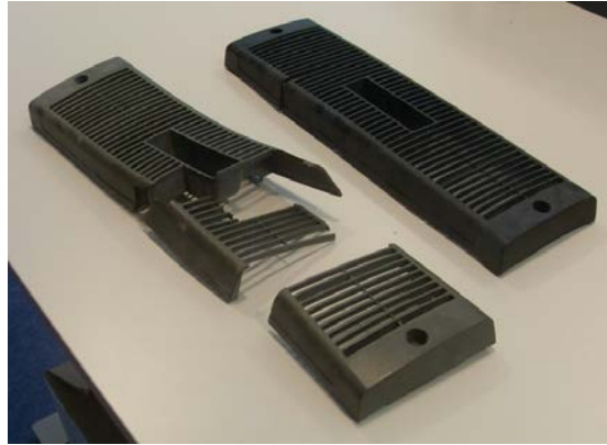
Figure 47. Fractured green and black PC/rPET covers. The green cover (on the left) was dropped onto the black cover (on the right), which fractured due to the impact.
