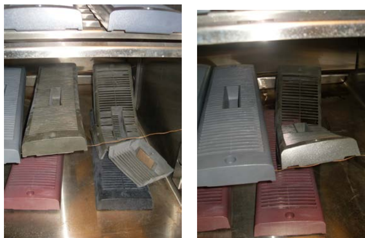
Figure 46. Fractured PC/rPET covers. The cover on the left fractured after 1500 h and the cover on the right fractured after 1530 h.
