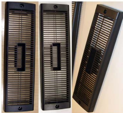
Figure 92. Visual inspection of rPC 65 covers after 0 (on left), 1000 and 2000 h in accelerated aging testing. Material maintained its appearance.
