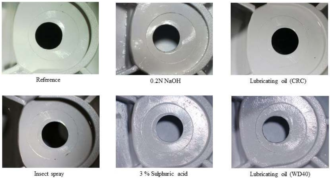
Figure 101. rPC 10 after chemical test. Photos were taken with macroscope. Objective magnification was 5.8x. Surfaces of the covers were wiped with water to remove residual chemicals.
