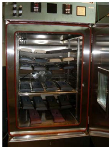
Figure 30. Test chamber for 85/85 accelerated aging test. 2 rear covers of each material were exposed to 85 °C and 85 % RH for 2 000 h.
