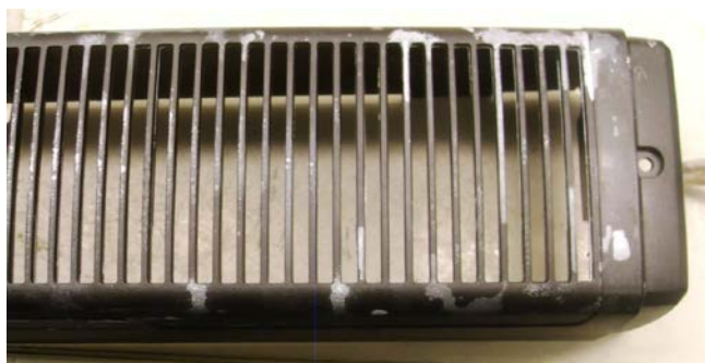
Figure 57. NaOH spots on the PC/rPET cover after the chemical test. Material under the NaOH layer was intact.
