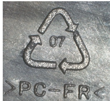
Figure 13. Recycling mark in a plastics product. Number 07 indicates that the plastic belongs to group 'other'. Additional marking informs that the material is flame retarded (FR) polycarbonate (PC).
