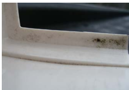
Figure 68. Dirt on the surface of PA 410 cover after 6 months outdoor exposure in Espoo.
