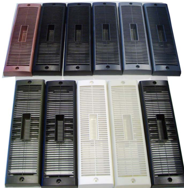
Figure 29. Samples of rear cover. Upper row from left to right: rPC 100 (red), rPC 100 (black), rPC 65, rPC 30, rPC 10 and vPC. Lower row from left to right: PC/rPET (green), PC/rPET (black), PA 410, PTT GF and rPC 30B.
