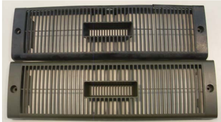
Figure 49. Deformation in the PC/rPET cover after 1500 h in accelerated aging testing. The black PC/rPET cover above was deformed due to hydrolysis. Below is a green PC/rPET cover which was not exposed to the test conditions.
