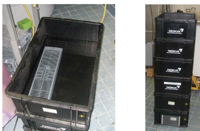
Figure 39. Immersion of rear covers. Plastic containers were filled with deionized water.
