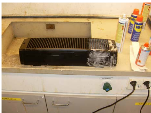
Figure 31. Configuration of the chemical testing: exposure by spraying and rubbing with cotton plug. Exposure times were 15 - 20 s.
