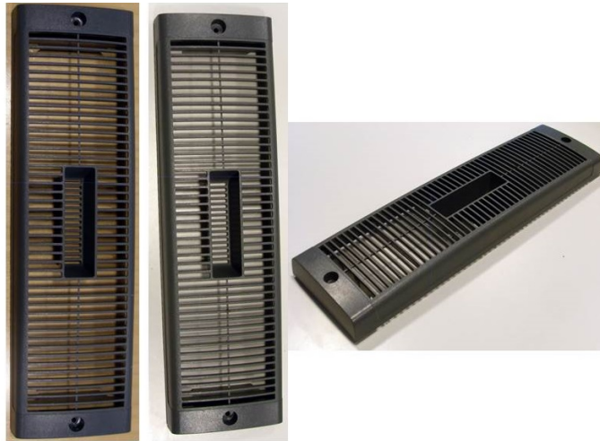
Figure 88. vPC covers in accelerated aging test after 0 (on left), 1000 and 2000 h. The appearance did not degrade during the test.
