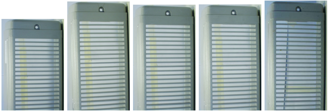
Figure 75. rPC 65 samples after 6 months outdoor exposure. Samples from left to right: an unexposed sample and the samples tested in Athens, Oulu, Espoo and Nairobi.
