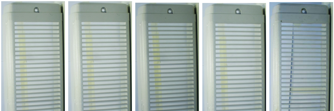
Figure 73. rPC 30 samples after 6 months outdoor exposure. Samples from left to right: an unexposed sample and the samples tested in Athens, Oulu, Espoo and Nairobi.
