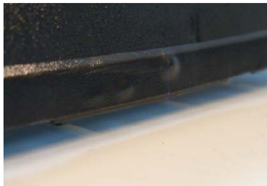
Figure 45. Bubble formation in PC/rPET covers in the accelerated aging testing after 190 h. Gas was trapped inside the material during moulding. When temperature was increased gases expanded which caused bubbling.
