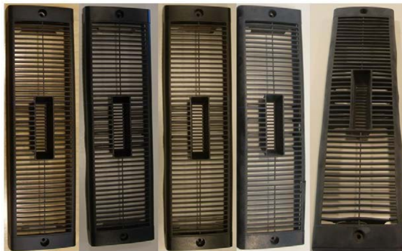
Figure 48. The colour change in a PC/rPET cover. Photos were taken with digital camera after 0 (on left), 500, 1 000, 1 500 and 2 000 h. Grey material layer formed on the surface after 1 500 h.
