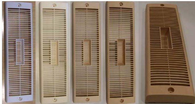
Figure 85. Colour change in PA410 in accelerated aging test. Photos were taken with digital camera after 0 (on left), 500, 1 000, 1 500 and 2 000 h.
