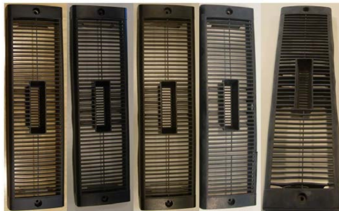
Figure 86. Colour change in PC/rPET cover in accelerated aging testing. Photos were taken with digital camera after 0 (on left), 500, 1 000, 1 500 and 2 000 h. Grey material layer was formed on the surface after 1 500 h.
