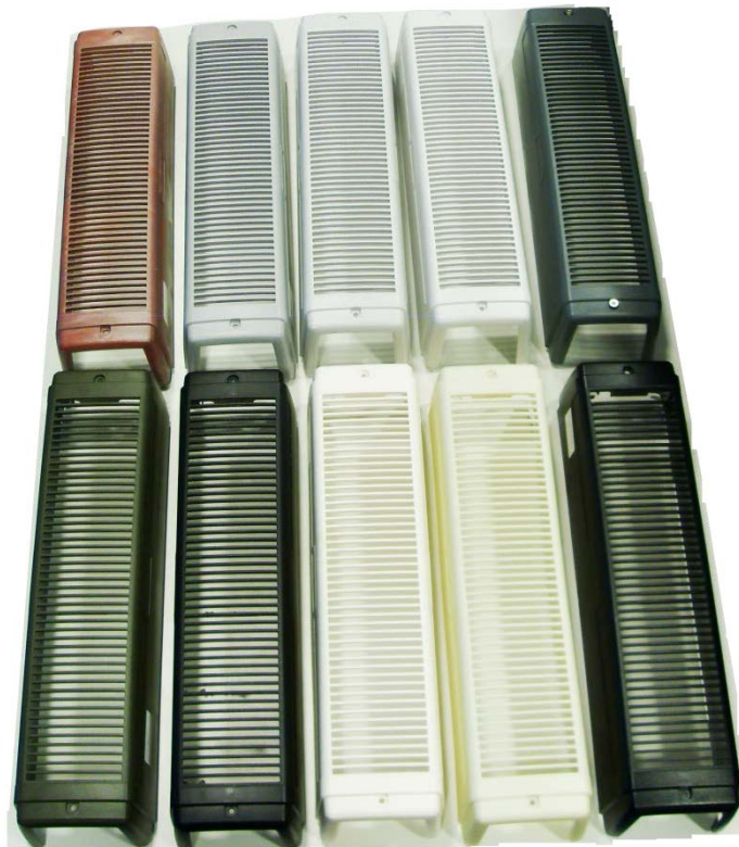
Figure 28. Samples of front covers. Upper row from left to right: rPC 100, rPC 65, rPC 30, rPC 10 and vPC. Lower row from left to right: PC/rPET (green), PC/rPET (black), PA 410, PTT GF and rPC 30B.
