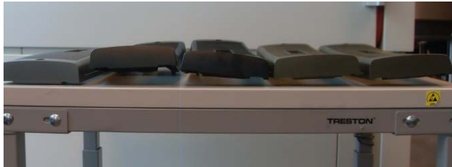
Figure 44. The deformation in PC/rPET covers after 190 h in the accelerated aging testing. The grey cover on the left is reference cover made from vPC.
