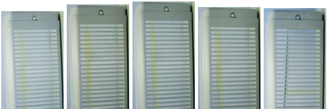
Figure 72. rPC 10 samples after 6 months outdoor exposure. Samples from left to right: an unexposed sample and the samples tested in Athens, Oulu, Espoo and Nairobi.
