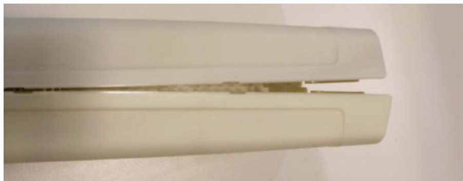
Figure 52. A PTT sample after the accelerated aging testing. The material became slightly brighter in the test. The cover above is tested in 85/85 conditions. The cover below is an untested sample.
