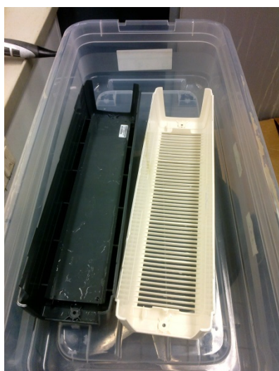
Figure 32. Exposed front covers in plastic containers. The containers were sealed with duct tape and the covers were kept in containers for 30 days.
