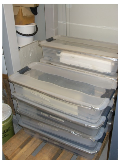
Figure 32. Exposed front covers in plastic containers. The containers were sealed with duct tape and the covers were kept in containers for 30 days.
