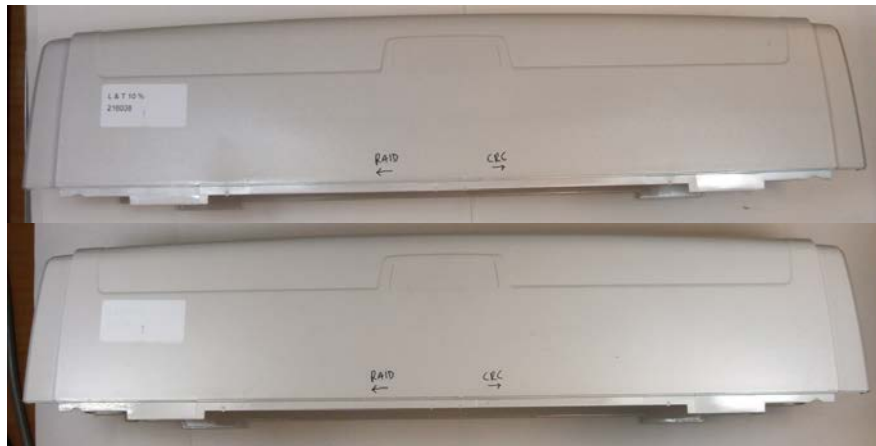
Figure 55. rPC 10 cover before (above) and after (below) insect spray and lubricating oil exposure. Insect spray (RAID) was sprayed on the left end of the cover.
