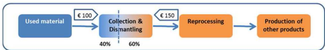
Figure 9. The principle of economic allocation in recycling. Environmental impacts from the collection and dismantling processes are divided between first and second life based on the economic values of virgin and recycled materials. (Lighthart & Ansems 2012)
