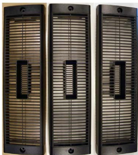
Figure 93. Visual inspection of rPC 100 cover after accelerated aging testing. Pictures are taken after 0 (on left), 1000 and 2000 h.
