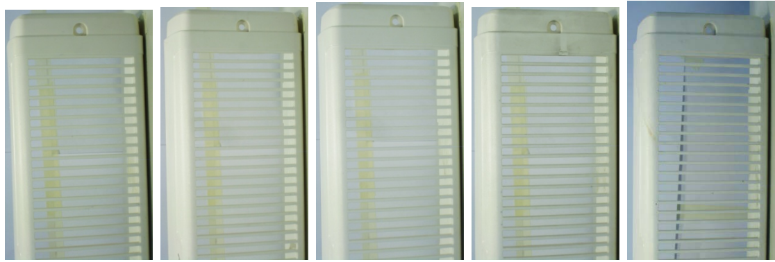
Figure 69. PA 410 samples after 6 months outdoor exposure. Samples from left to right: an unexposed sample and the samples tested in Athens, Oulu, Espoo and Nairobi.
