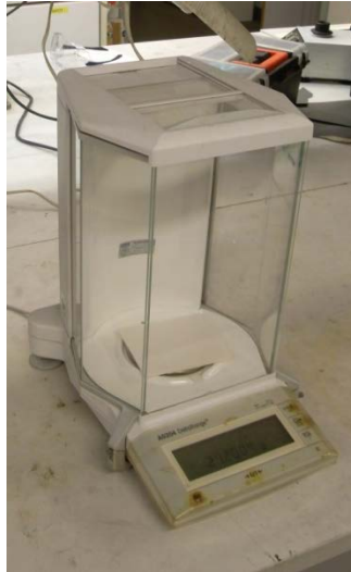
Figure 37. The weighing of a sample during the water absorption testing. The weighing was performed before and after drying and during the test until equilibrium was reached.
