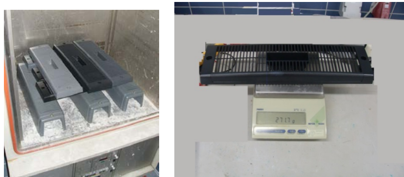
Figure 38. Drying and weighing of rear covers for the water absorption test. The covers were dried at 39 °C for 4 h. The covers were weighed before and after drying and every 24 h during the immersion.
