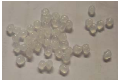
Figure 16. Plastic waste is processed into small granulates with size of 4x4x5 mm. Granulates in the photo are PP.
