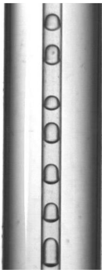
Figure 8. Elongated confined bubbles in a small scale tube [13]
