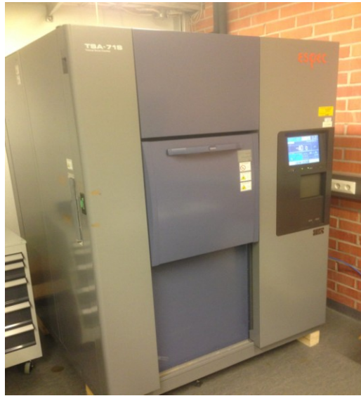
Figure 31: ESPEC TSA-71S thermal shock chamber which was used to do thermal cycling test.
