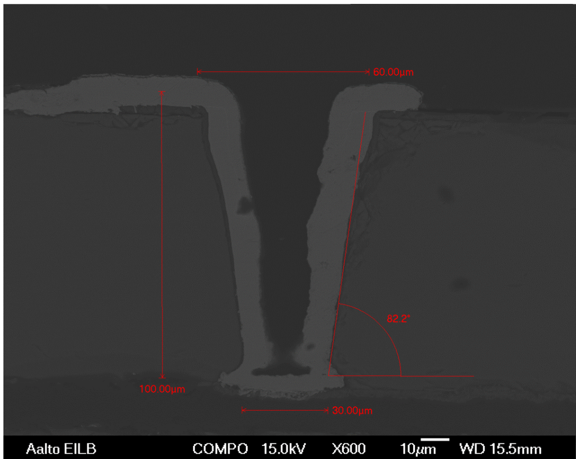
Figure 43: Backscatter electron image of a single via with dimensions values.
