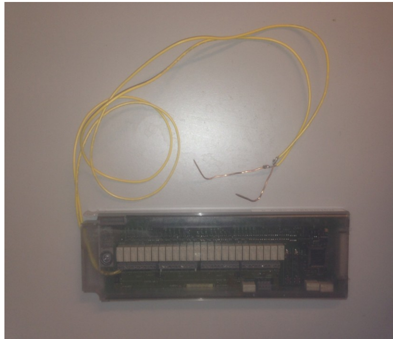
Figure 30: Self-made probes attached to Agilent 34901A 20-Channel Armature multiplexer.
