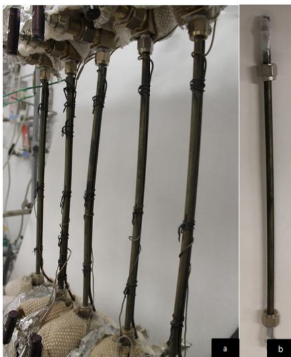
Figure 5.1: Reactor tubes. (a) Reactors installed in the set up, including resistors and thermocouples. (b) Single reactor.
