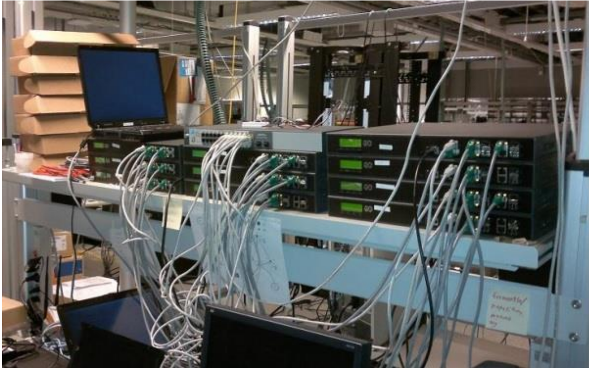
Figure 5.11: Wireless mesh network with Lanner MR-730 units in NSN Mobile Backhaul Advanced laboratory.
