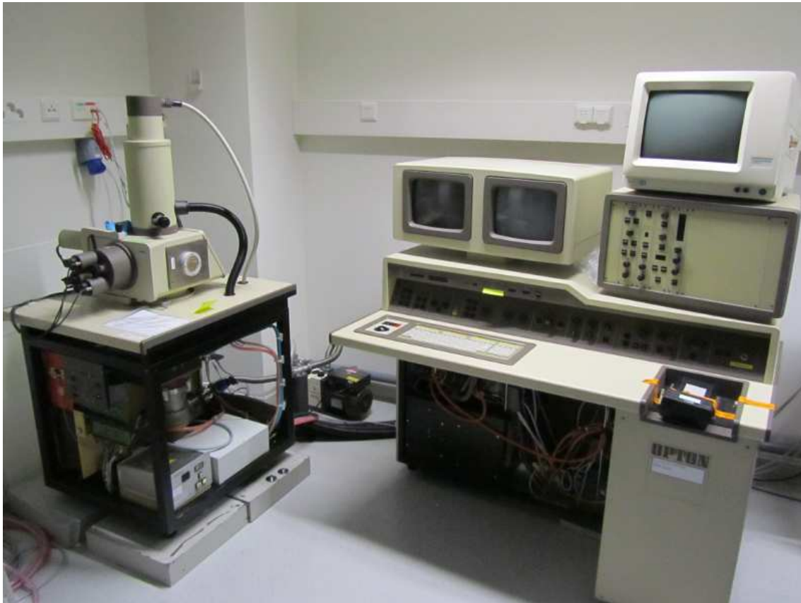
Figure 40: DSM 950 (ZEISS/Opton) scanning electron microscope consists of separate microscope and operating modules. The controls of the vacuum system are located in the front side of the microscope module. The controls of the electron beam are located in the operating module.
