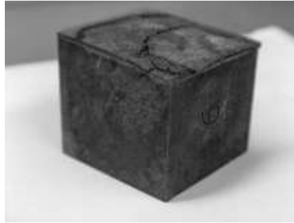
Figure 62 Sample's cracked surface after 950°C austenitising and 350°C austempering.
