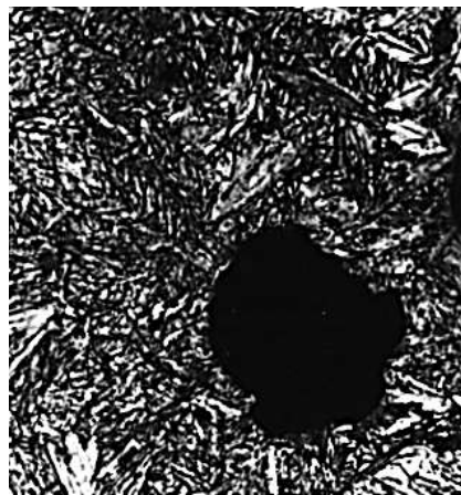
Figure 13 Micrograph of martensitic quenched ductile iron. \sim 880\times [19]
