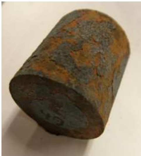
Figure 56 Sample GJS-500-7 after austenitisation at 860°C.
