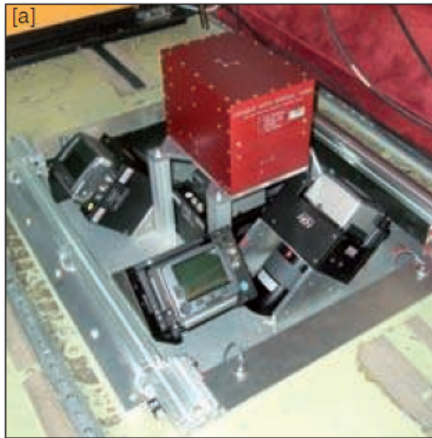
Figure 12: An IGI Penta-DigiCAM system with a single vertical camera (equipped with an f=28 mm lens) in the centre. It is flanked by the four tilted cameras (each with an f=150 mm lens) that generate the surrounding oblique images of the ground. An AEROcontrol IMU unit has been mounted directly over the vertical camera (Petrie, 2009).
