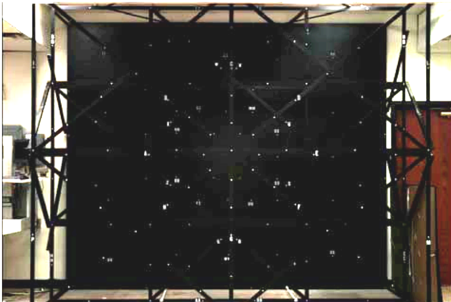
Figure 6: Calibration cage (Wang et al., 2008)
