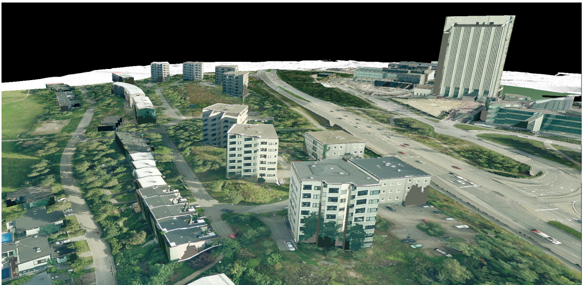
Figure 25: The 3D model made with TerraPhoto, TerraScan and TerraModeler ©Tomi Rosnell, FGI 2014.
