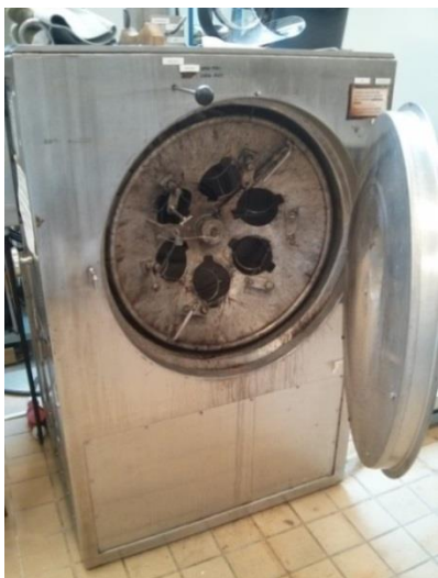
Figure 25. Air bath digester used for preliminary tests, A- and EOP-stages.
