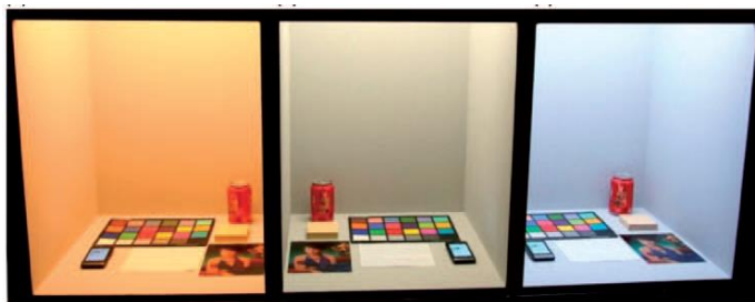
Figure 1. The booth with a different light source in each section: LED luminaires in the left and right, and fluorescent lamp luminaire in the middle
