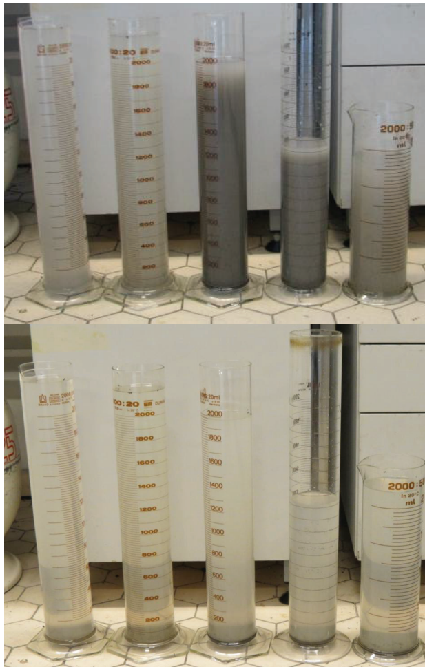
Figure 6. Gravitational columns before and after 72 h precipitation stage. The three columns on the left are from the first container and the two columns on the right from the second container.
