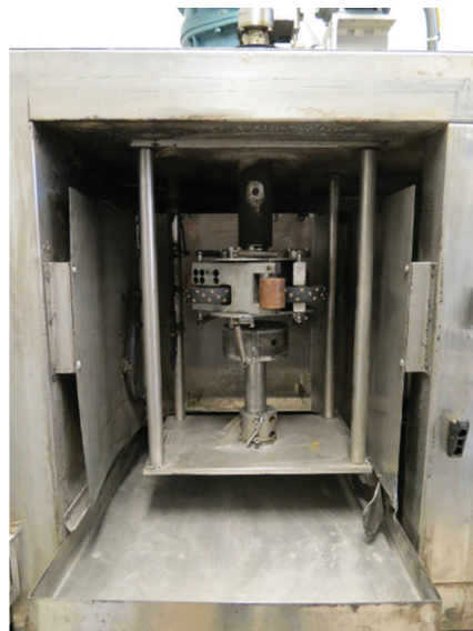
Figure 3. Cleaned SRK chamber for abrading the fines from SRK-samples.
