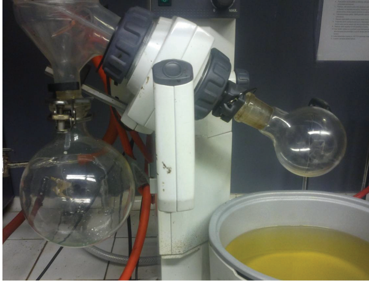
Figure 13. The apparatus used for the execution of reactions of abraded fines (SRK-test) with deicing solutions.
