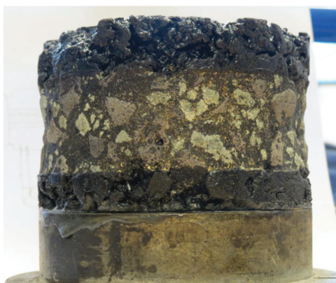
Figure 2. Left VT4 mixture Sample 3 (with OKTO-aggregate) after SRK abrasion and right results of Prall testing of the same mixture.
