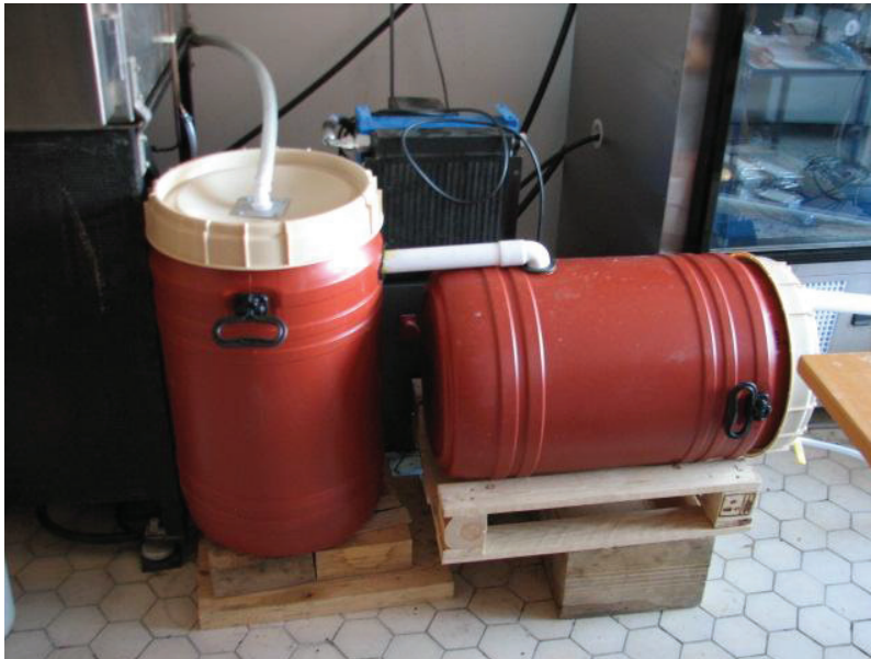
Figure 4. Waste water collecting system – a) schematic representation, where red arrows indicate assumed waste water flow, b) the actual setup.
