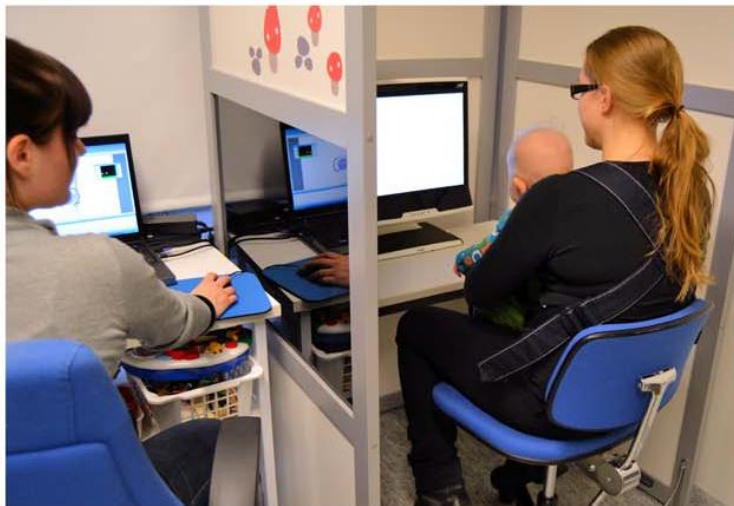
Figure 4. Eye tracking setup. The photograph shows the laboratory setup where infant is placed into a baby carrier attached to the chest of the caregiver (right), and the experimenter (left) is sitting behind a light wall with one-way transparency (not visible on the photograph) that allows observation of the infant during the test. The figure is adopted from Ahtola et al. (2014).
