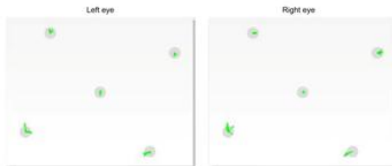
Figure 3. Eye tracker calibration results. Example screenshot from a calibration session demonstrating how Tobii Studio software shows the offset of gaze during calibration procedure. The figure is adopted from Ahtola et al. (2014).
