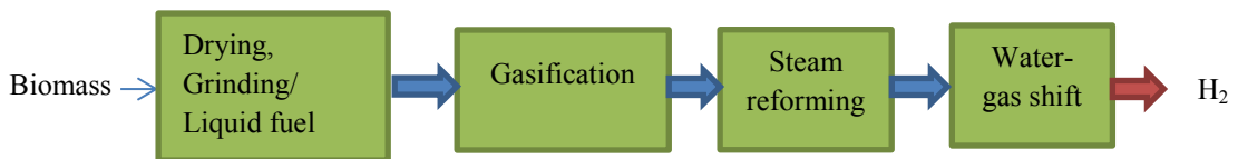
Figure 6. Block diagram of biomass gasification process. (Patronen, 2011)
