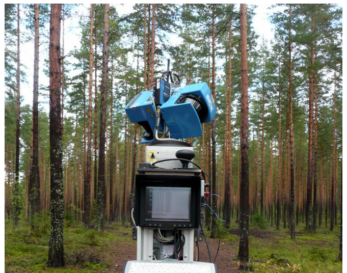
Fig. 1. Measured pine forest and the rotating 3D laser scanner on an all-terrain vehicle driving through the forest while measuring.
