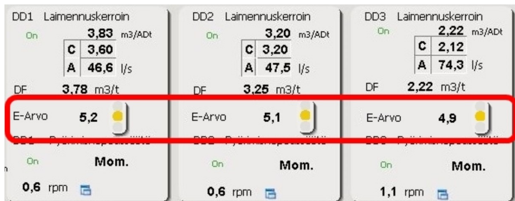
Figure 26. The E-value and the efficiency traffic lights on the operation monitor of the upper level control.
