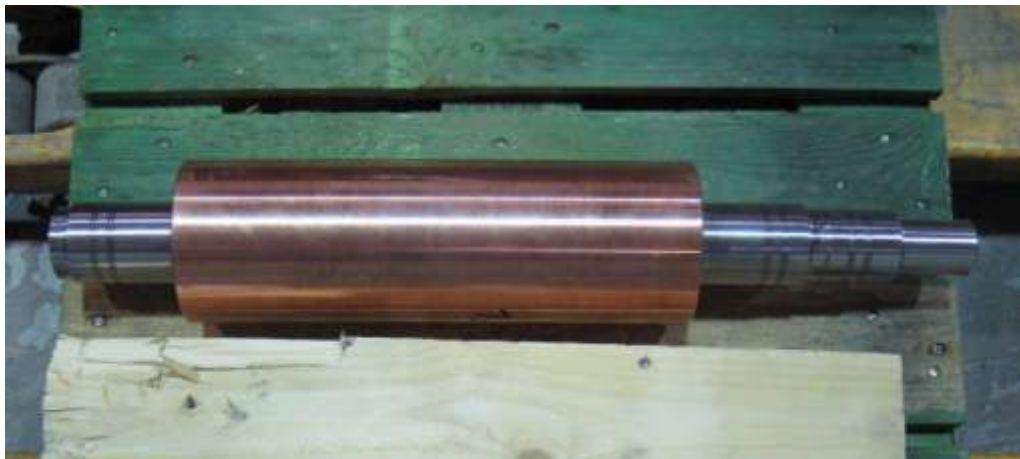
Figure 28. Prototype rotor copper coated by explosion welding.
