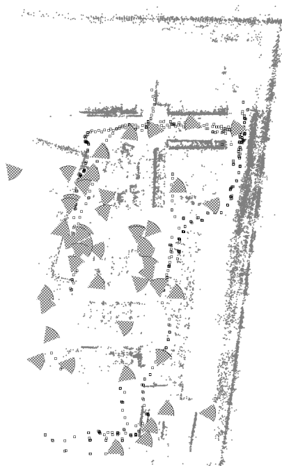
Figure 7.5: Successfully located images and their viewing directions (marked as patterned shapes)
