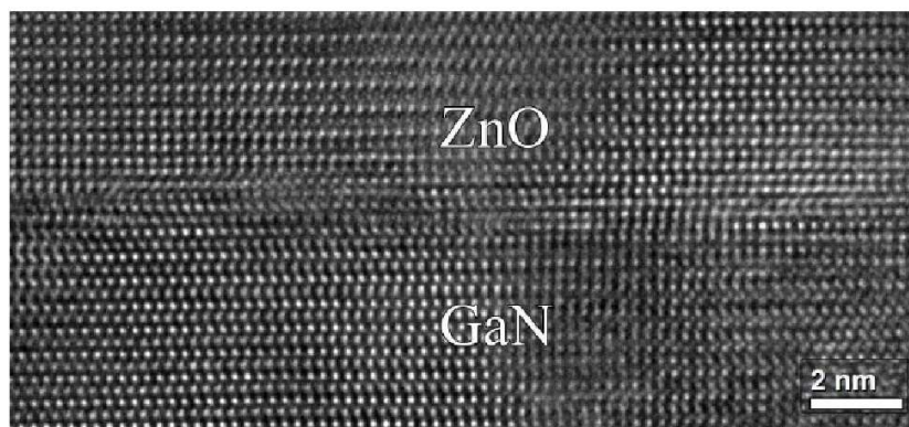
Figure 6.4: TEM image of the interface of epitaxial ZnO on GaN.[101]
