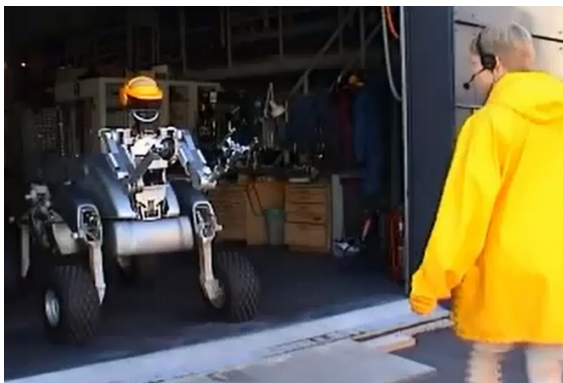
Figure 3.2: User identification Workpartner: The robot Workpartner identifies the human user based on color coded clothes.
