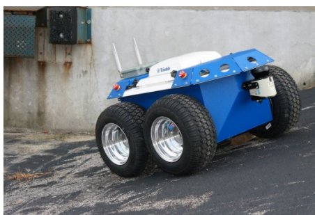
Figure 2.5: The autonomous all-terrain vehicle research platform Seekur Jr. [21].
