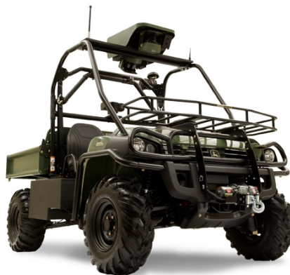
Figure 2.1: The R-Gator based on the John Deere XUV utility vehicle [9].
