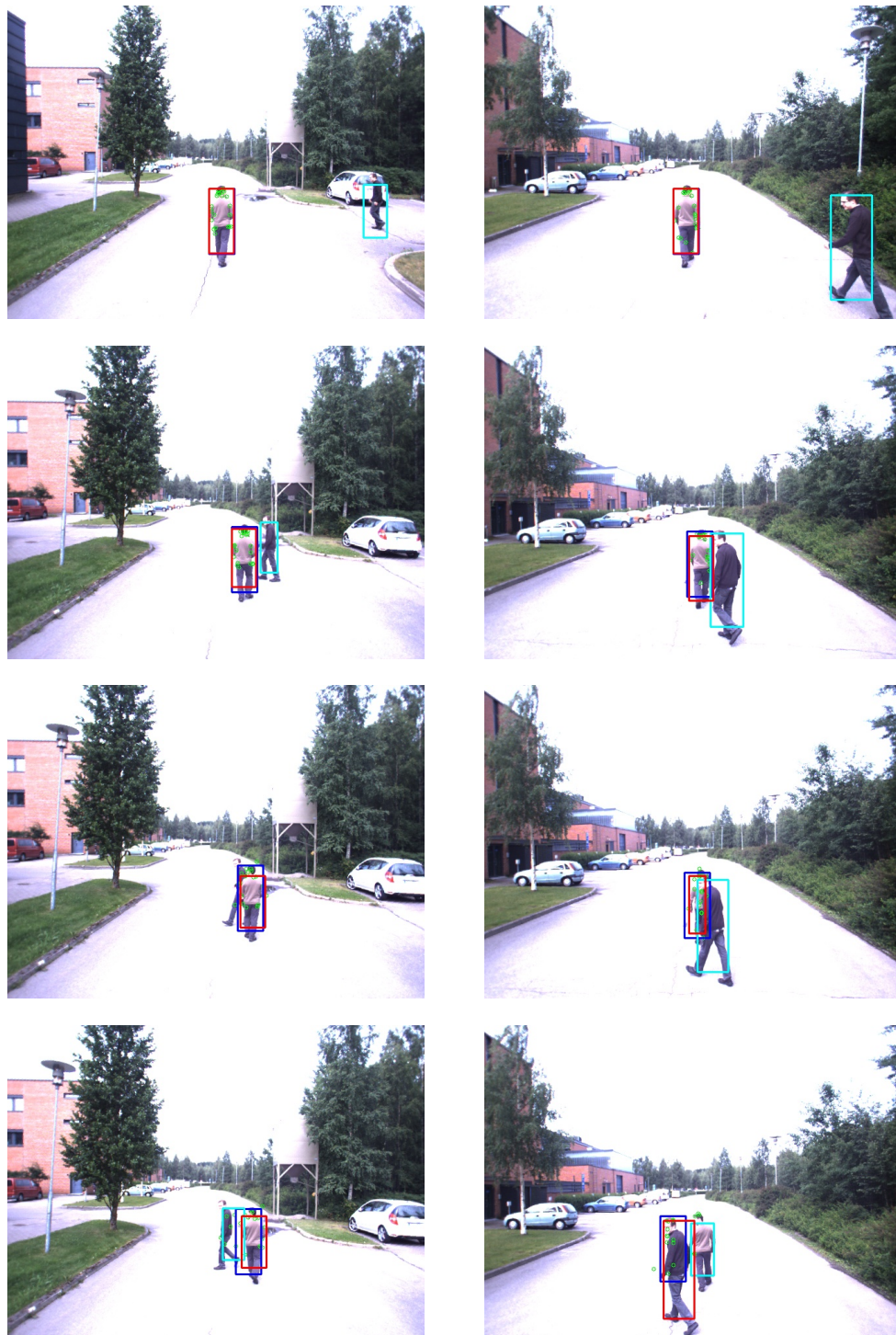
Figure 7.9: Two different crossing situations: On the left side, the user's path is crossed by another person in front of the user, while on the right side, the crossing happens between the user and the car. The user is marked with a red box, while other people that are detected by the LIDAR are indicated with a cyan box. The blue box shows the CMT image tracking result. The green circles show the tracked features.
