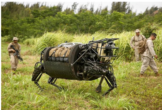
Figure 2.3: The Legged Squad Support System during military tests on Hawaii in 2014 [16].
