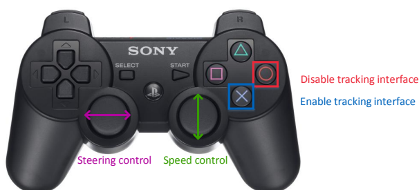
Figure 6.3: The PS3 controller user interface: The X-button activates the tracking interface, the O-button deactivates the tracking interface, the right analog-stick controls the speed and the left analog-stick controls the steering angle.
