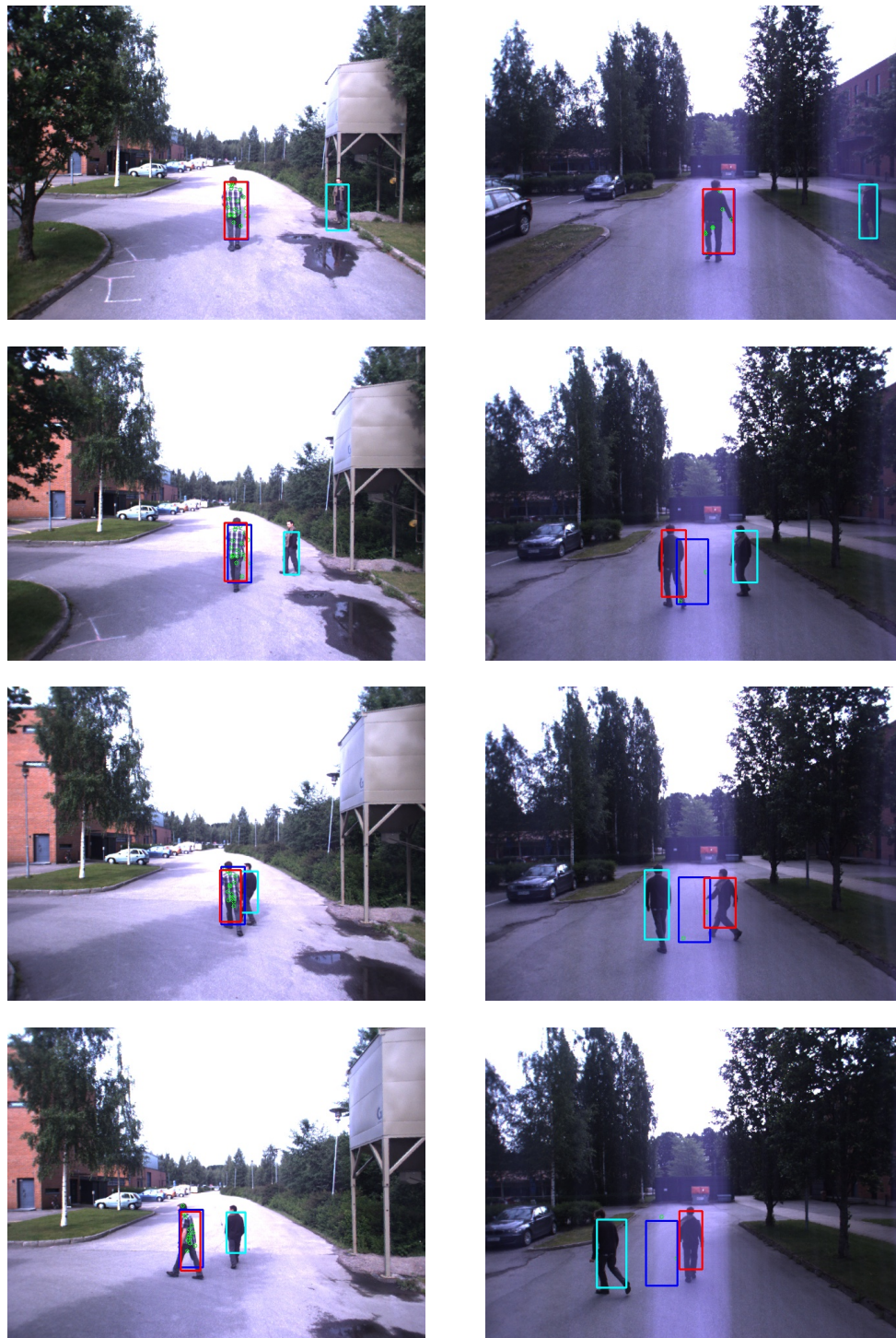
Figure 7.7: False Crossing in different situations. The scenes in the left column are well illuminated and the user wears clothes with a high contrast. Conversely, the scenes in the right column are badly illuminated and the user wears low-contrast clothes. The user is marked with a red box, while other people that are detected by the LIDAR are indicated with a cyan box. The blue box shows the CMT image tracking result. The green circles show the tracked features.
