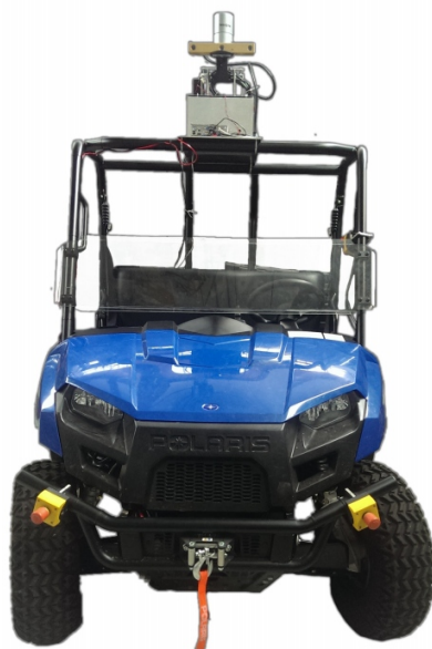
Figure 5.4: The Polaris Ranger ATV with mounted Velodyne HDL-32E, Bumblebee XB3 and perception computer.
