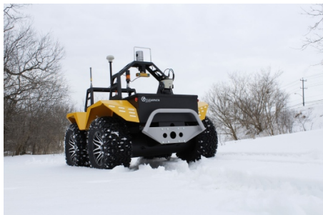
Figure 2.4: The autonomous all-terrain vehicle research platform Grizzly [22].
