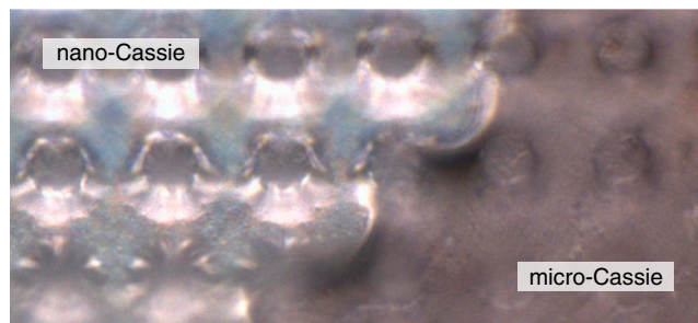
Fig. S2. An optical micrograph of a micro-Cassie/nano-Cassie boundary. The sample is tilted by 22° so that horizontal water-air interfaces do not reflect incident light to the objective. Consequently interfaces with a nonhorizontal slope appear brightest. Due to this, the air pockets at the bases of the posts are shown clearly. It is also obvious that the nano-Cassie region is much brighter overall due reflections from the interfaces between the air pockets and water. Because of the tilt and the shallow depth of field of the objective, only one row of posts is in focus in the image.
